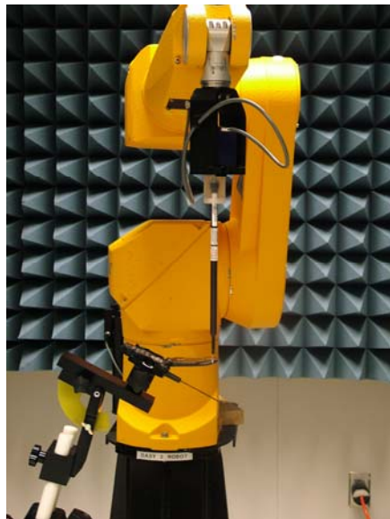
DUT test setup with 10mm spacing
