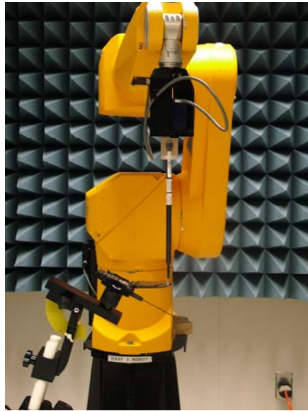
DUT test setup with 10mm spacing
