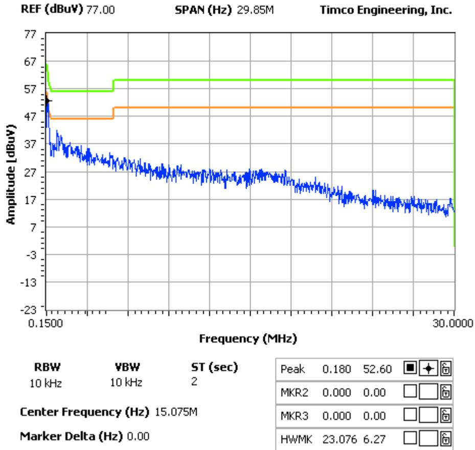
**Figure 6-7. Mains Voltage with Peak and AverageDetector.**
