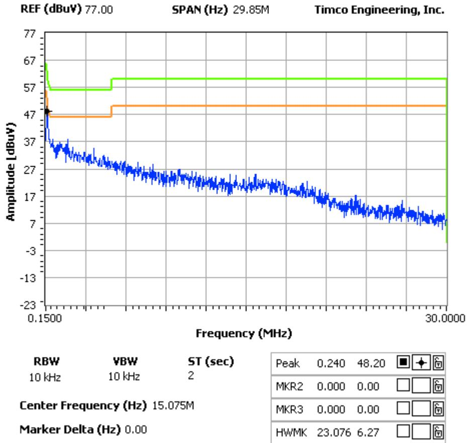
**Figure 6-8. Mains Voltage with Peak and AverageDetector.**
