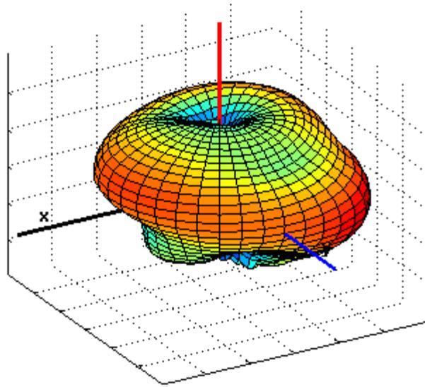
**Figure 6-6. GSM PCS antenna radiation pattern.**
