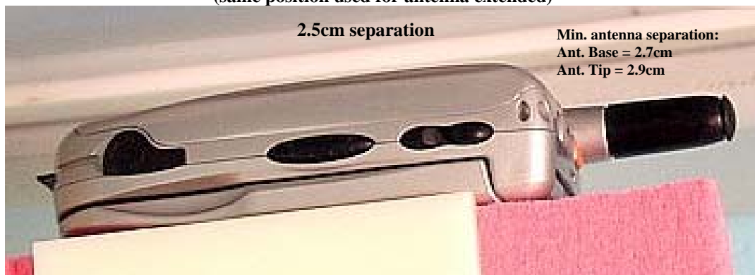
Figure 8. Assessment @ the body DUT back 2.5cm separation distance from flat phantom. (same position used for antenna extended)
