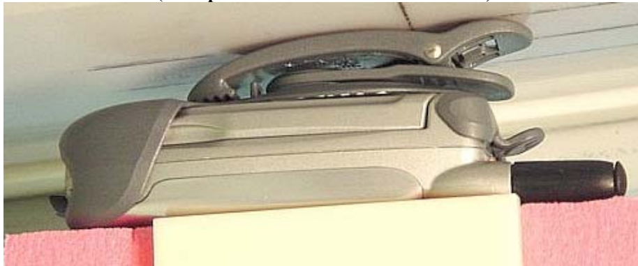
Figure 6. Assessment @ the body DUT with body worn accessory model NNTN4682A against the flat phantom. (same position used for antenna extended)
