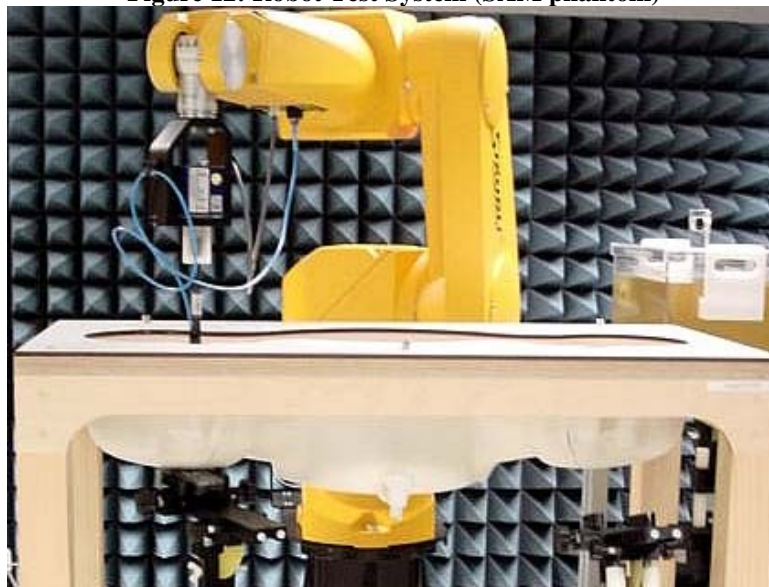
Figure 12: Robot Test System (SAM phantom)
