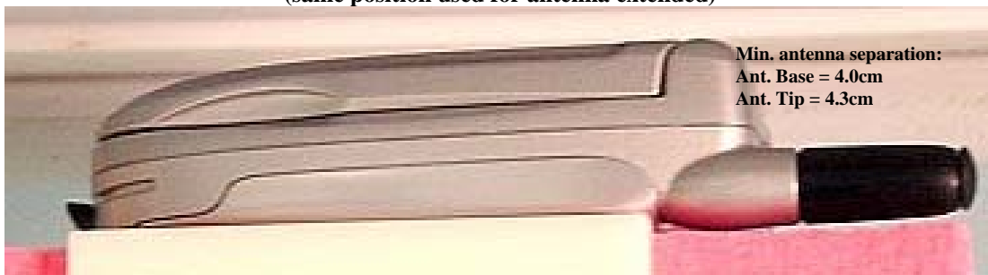
Figure 7. Assessment @ the body DUT front 2.5cm separation distance from flat phantom. (same position used for antenna extended)
