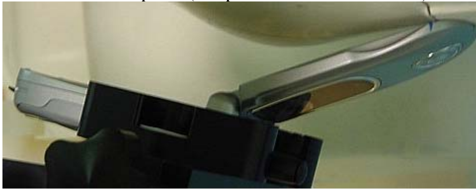
Figure 4. Assessment @ the Right ear DUT in Cheek touch position (same position used for antenna extended)
