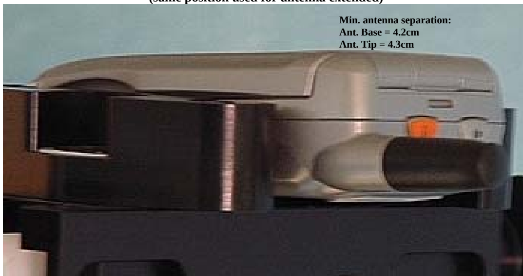
Figure 10. Assessment @ Face DUT front 2.5cm separation distance from flat phantom (flip closed). (same position used for antenna extended)
