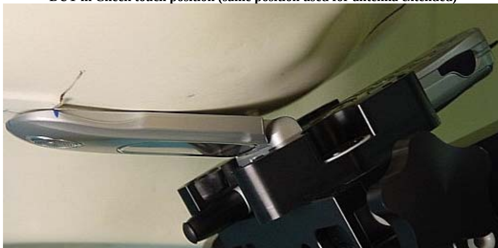
Figure 5. Assessment @ the Right ear DUT in 15° tilt position (same position used for antenna extended)
