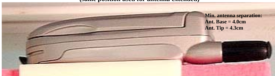
Figure 8. Assessment @ the body DUT back 2.5cm separation distance from flat phantom. (same position used for antenna extended)
