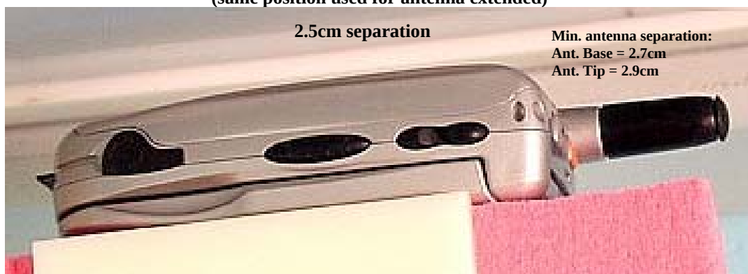
Figure 8. Assessment @ the body DUT back 2.5cm separation distance from flat phantom. (same position used for antenna extended)
