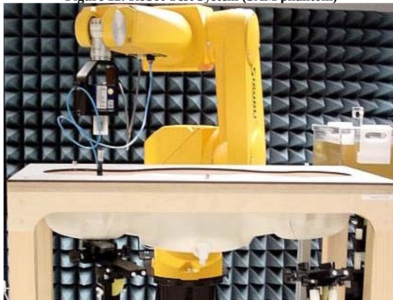
Figure 12: Robot Test System (SAM phantom)
