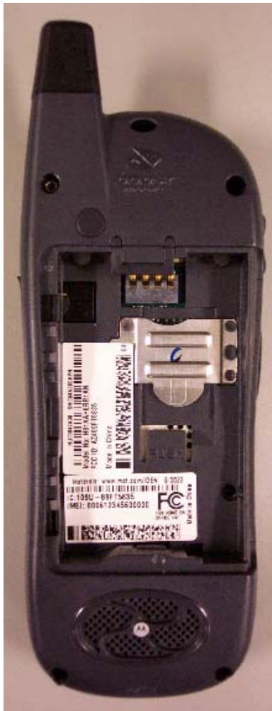
Photograph 1.1: Location of label on back of unit's housing (battery cover removed).
