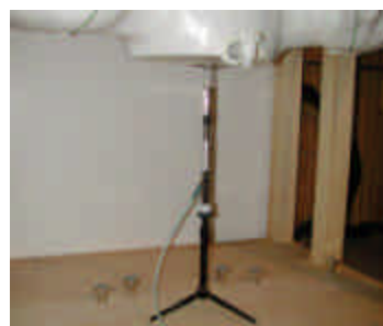
Figure 12.1 Dipole Validation Test Setup
