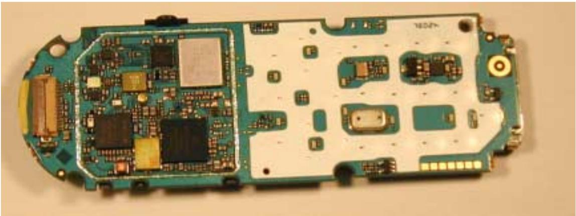
**Figure 9-5. Internal photo of electronic assembly with shields removed.**
