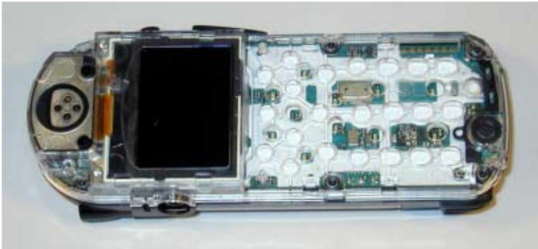
**Figure 9-3. Internal photo showing the keypad and display.**
