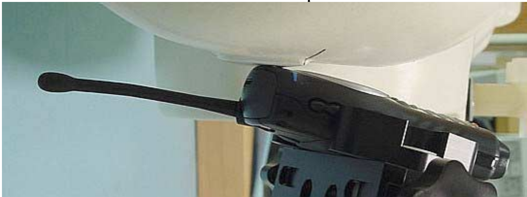
Figure 4. Assessment @ the Right ear. DUT in 15° tilt position.
