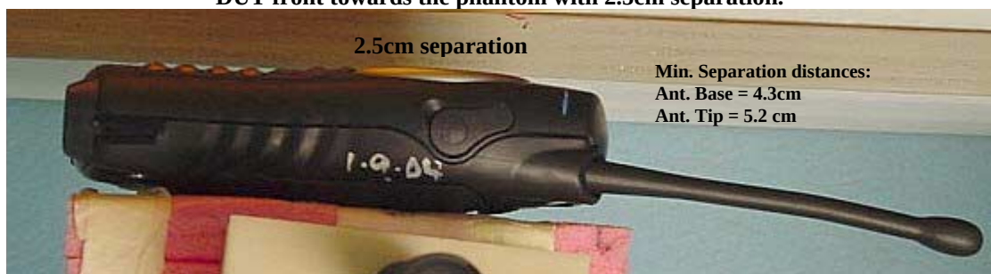
Figure 10: Robot Test System (Flat Phantom)
