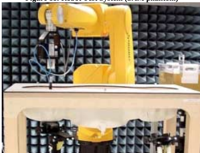
Figure 11: Robot Test System (SAM phantom)
