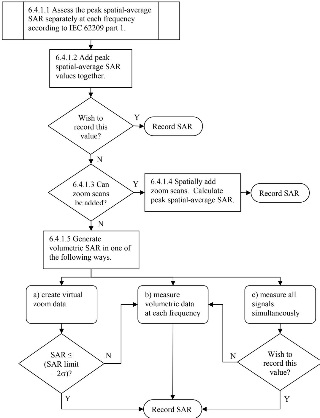
**Fig. 6.4.2. Flow chart of the process of section 6.4.**
