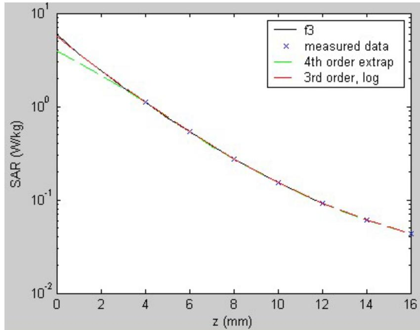
**Fig. 3: Curve fitting of  $f_3$  using two methods: 4<sup>th</sup> order polynomial fit to SAR and 3<sup>rd</sup> order polynomial fit to  $\log_{10}(\text{SAR})$ .**
