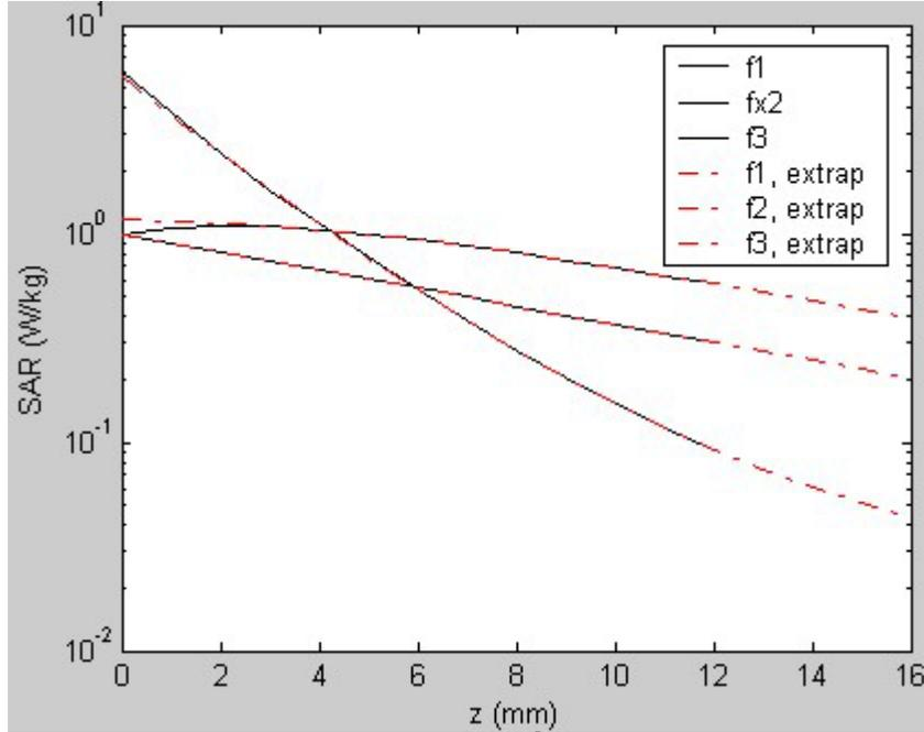
**Fig. 4: Curve fitting of  $f_1, f_{x2}$  and  $f_3$  using a 3<sup>rd</sup> order polynomial fit to  $\log_{10}(\text{SAR})$ .**
