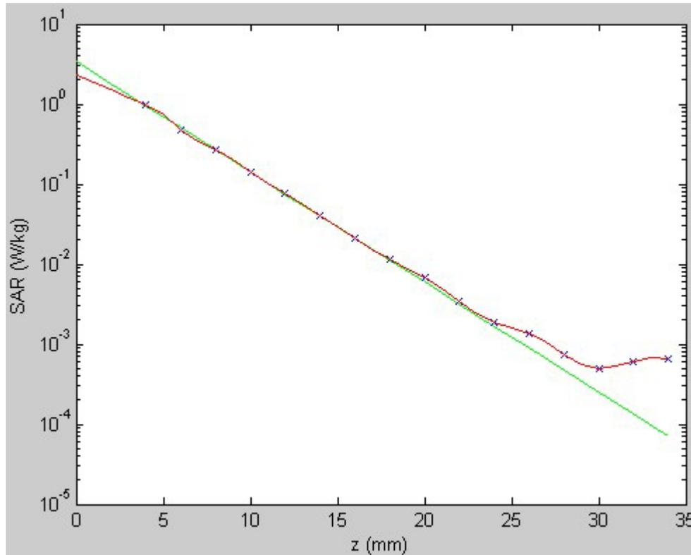
**Fig. 1: SAR distribution in the z direction (16 points). Blue crosses represent measured data. Red line represents data after 4<sup>th</sup> order polynomial extrapolation and spline interpolation. Green line represents exponential fit.**
