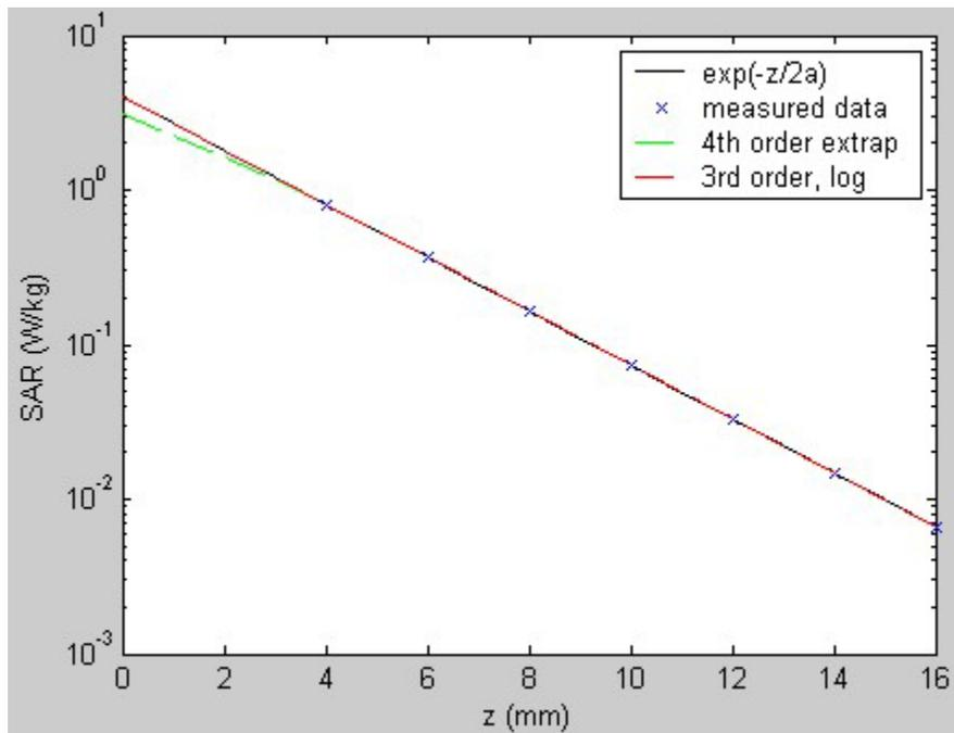
**Fig. 2: Curve fitting of  $4 \cdot \exp(-z/2a)$  using two methods: 4<sup>th</sup> order polynomial fit to SAR and 3<sup>rd</sup> order polynomial fit to  $\log_{10}(\text{SAR})$ .**
