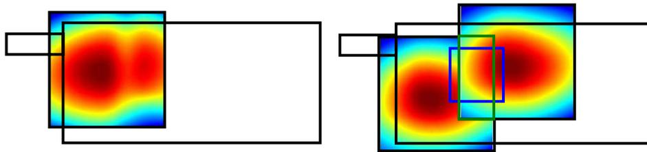
**Fig. 6.4.1: Two examples showing the zoom scans of a handset at two different frequencies, where the zoom scans overlap completely (left) or overlap slightly (right, overlap area shown in green) but not enough to contain the entire averaging volume (shown in blue).**
