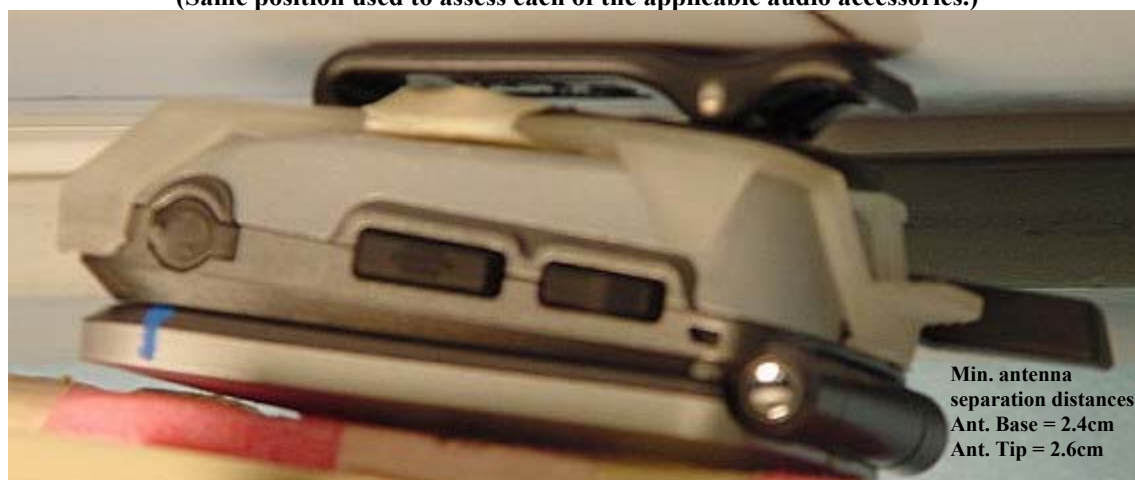
Figure 7. Assessment @ Body DUT w/ holster model NNTN5444A against the flat phantom (Same position used to assess each of the applicable audio accessories.)
