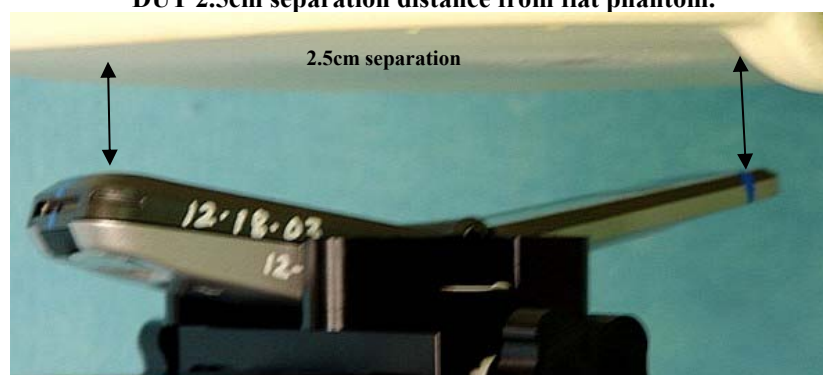
Figure 6. Assessment @ the Face; flip open DUT 2.5cm separation distance from flat phantom.
