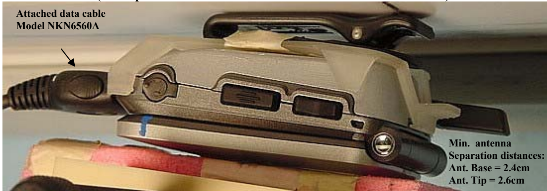
Figure 9. Assessment @ the Body DUT w/ belt clip model NTNN5159A. (Same position used w/ audio accessory model NNTN4620A attached)
