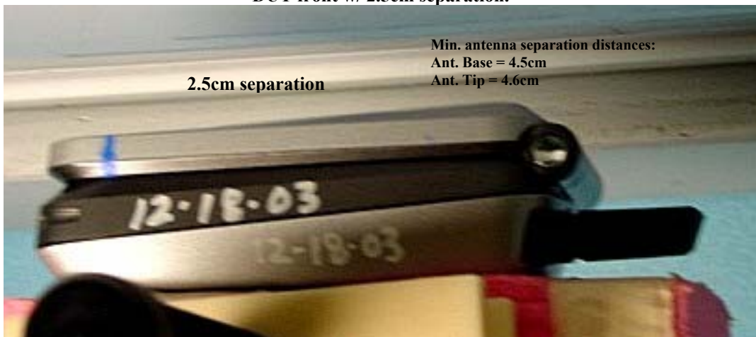
Figure 10. Assessment @ the Body DUT front w/ 2.5cm separation.
