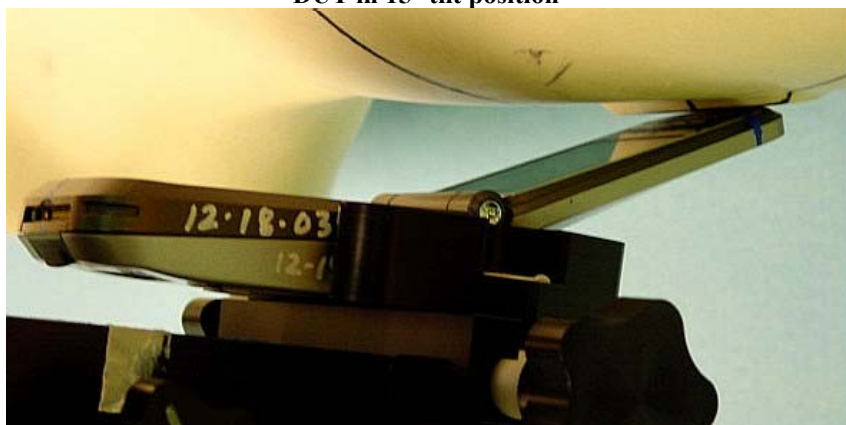
Figure 3. Assessment @ the Right ear DUT in Cheek touch position;
