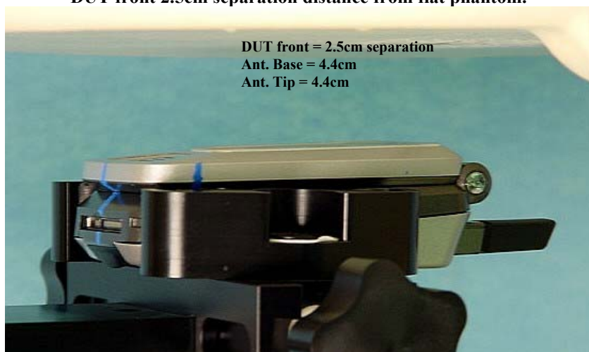
Figure 6. Assessment @ the Face; flip open DUT 2.5cm separation distance from flat phantom.
