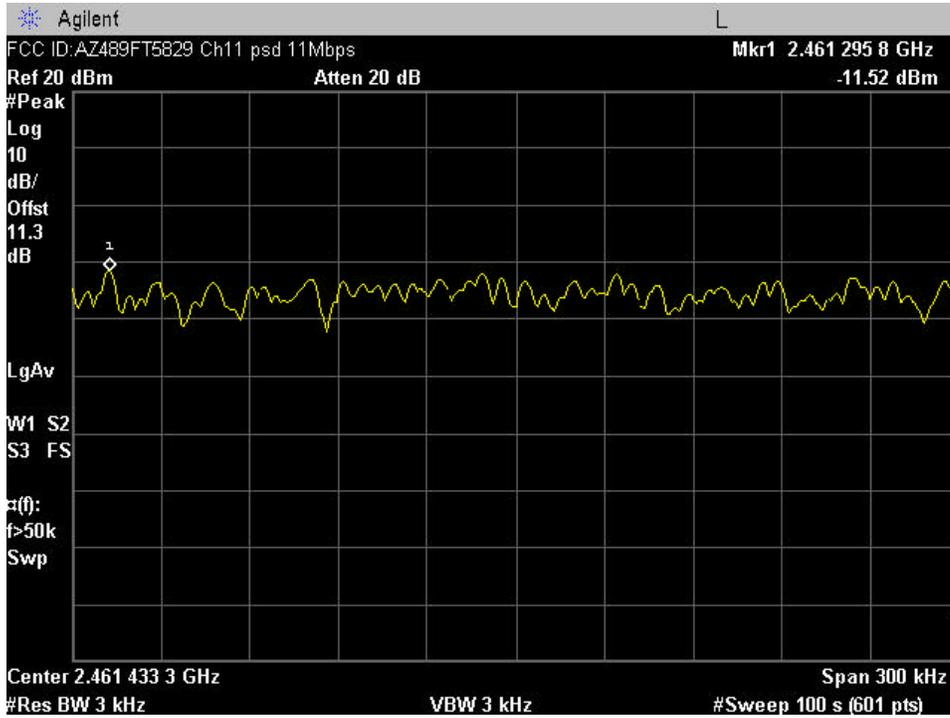
Plot A-12. Max. Power Density Plot – Ch. 11
