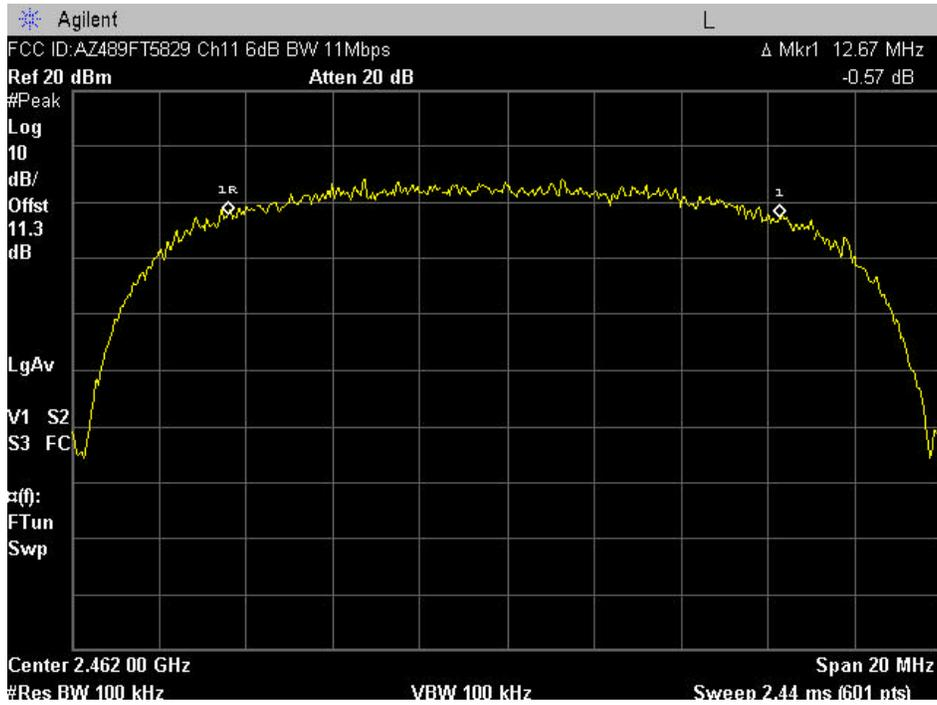
Plot A-3. 6dB Bandwidth Plot – Ch. 11
