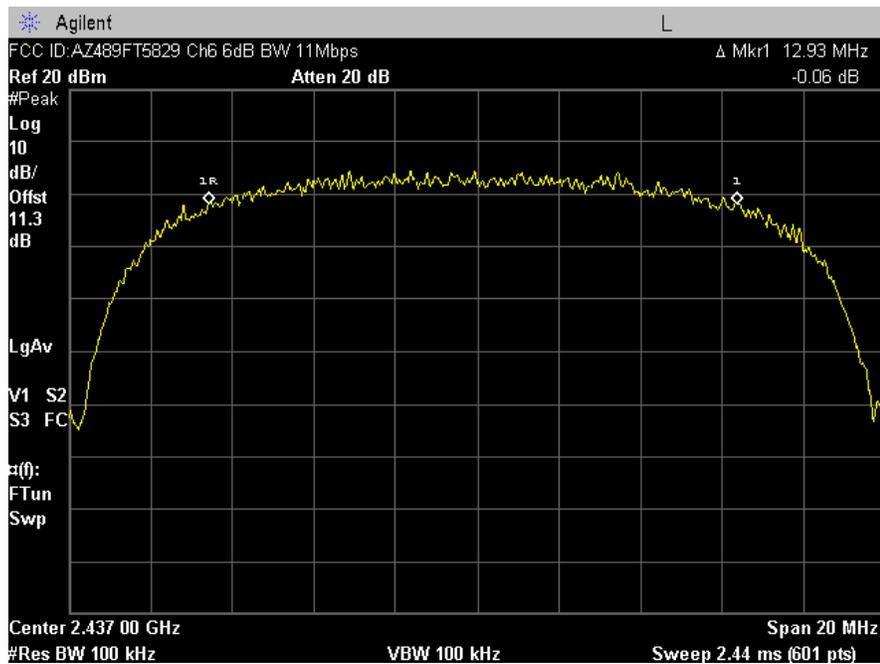
Plot A-2. 6dB Bandwidth Plot – Ch. 06
