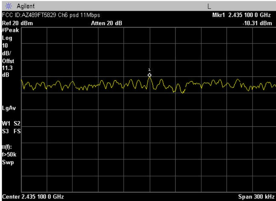
Plot A-11. Max. Power Density Plot – Ch. 06
