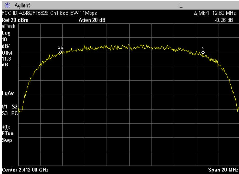
Plot A-1. 6dB Bandwidth Plot – Ch. 01
