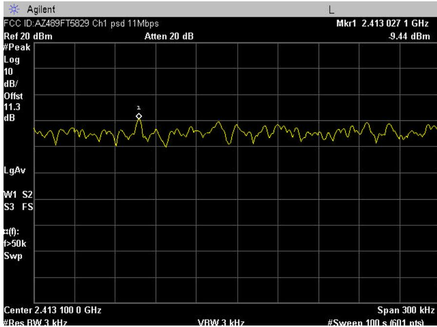
Plot A-10. Max. Power Density Plot – Ch. 01
