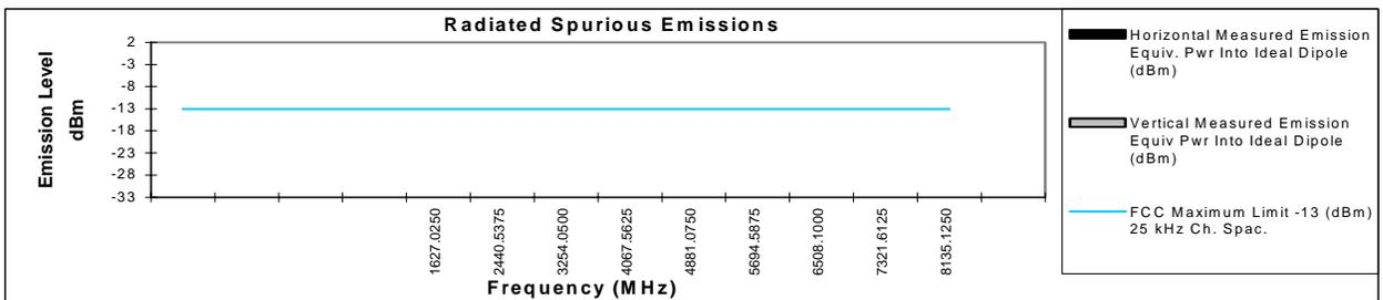
\* Indicates the spurious emission was less than -33dBm or could not be detected due to noise limitations or ambients.
