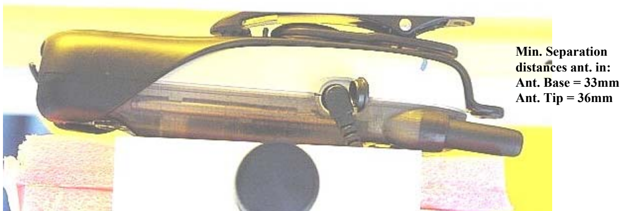
Figure 9. Assessment @ the Abdomen; DUT front 2.5cm separation. Similar position used for DUT back 2.5cm from phantom
