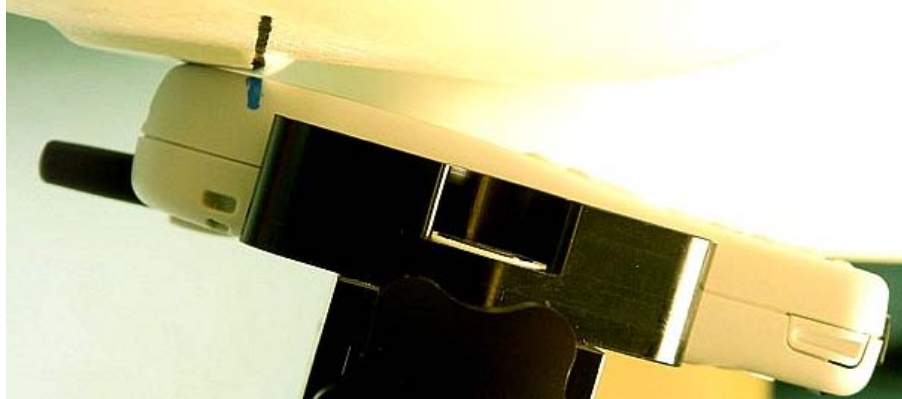
Figure 5. Assessment @ the Right ear; 15° tilt position; with antenna retracted. Same position used for antenna extended.
