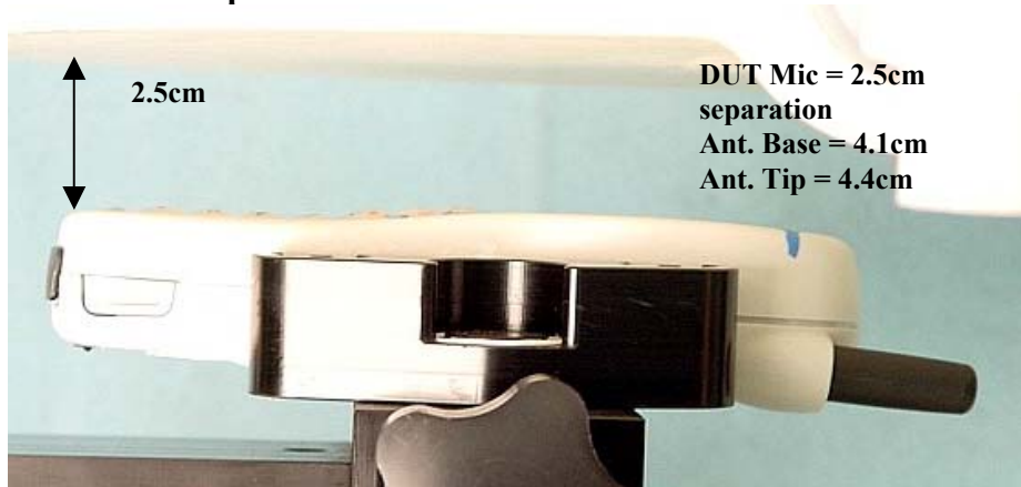
Figure 6. Assessment @ the Face; DUT microphone 2.5cm separation distance from flat area of SAM phantom
