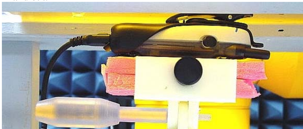
Figure 7. Assessment @ abdomen; DUT w/ carry case model NNTN4681A against the flat phantom and attached data cable model NKN6544B. Same position used to assess data cable models NKN6540A, NNTN4007A, NNTN4049A, NNTN4877A w/ antenna in and out.
