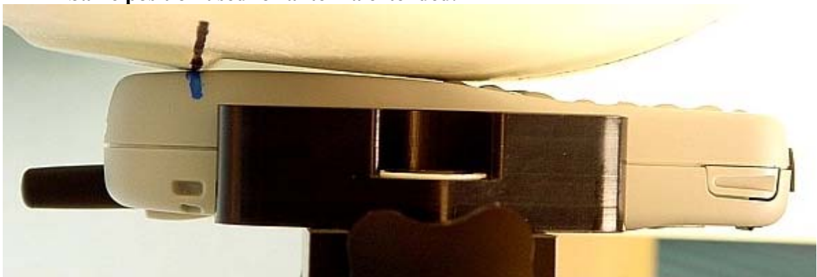
Figure 4. Assessment @ the Right ear; Cheek touch position; with antenna retracted. Same position used for antenna extended.
