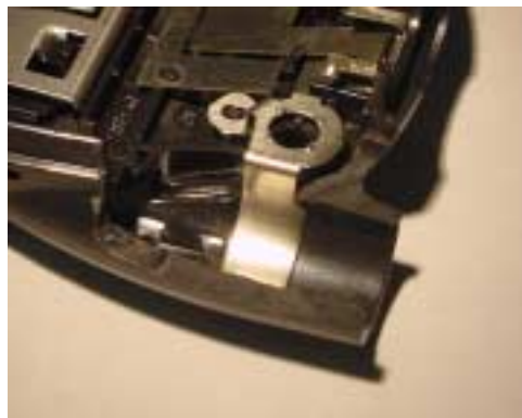
Figure 9-4. Photograph of original i85s/i55sr antenna clip (antenna boss removed for clarity).
