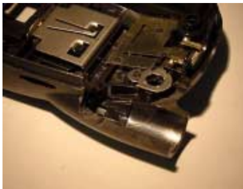
Figure 9-3. Photograph of i88s/i58sr antenna clip (antenna boss removed for clarity).
