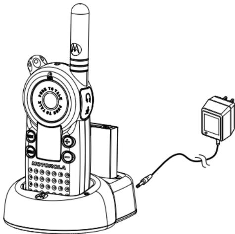
The drop-in charger will also sequentially charge a spare SNN5571 Li Ion battery. The spare battery will not begin to charge until the radio battery is fully charged. Both batteries will charge in approximately 2 to 6 hours.
