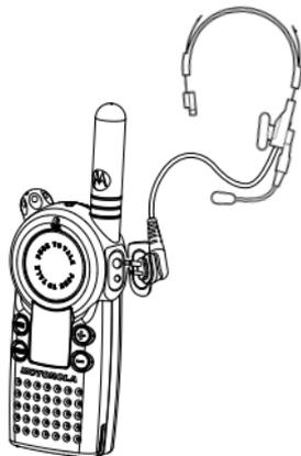
6. To transmit, speak into the accessory microphone. To receive, stop talking. To disable VOX operation, press **Push to Talk** or remove the audio accessory.
