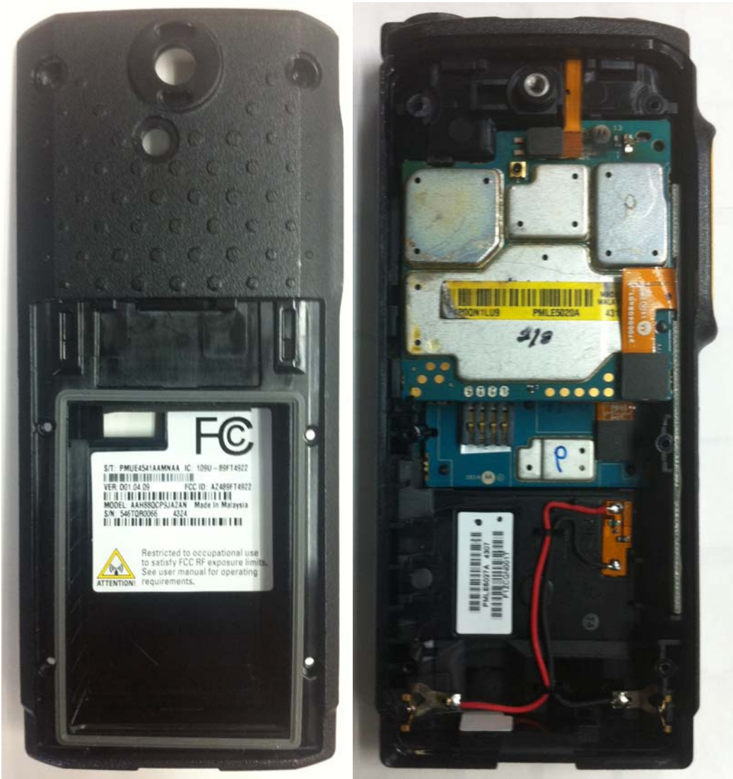
PCB board with chassis and housing for Display model (Bottom)
