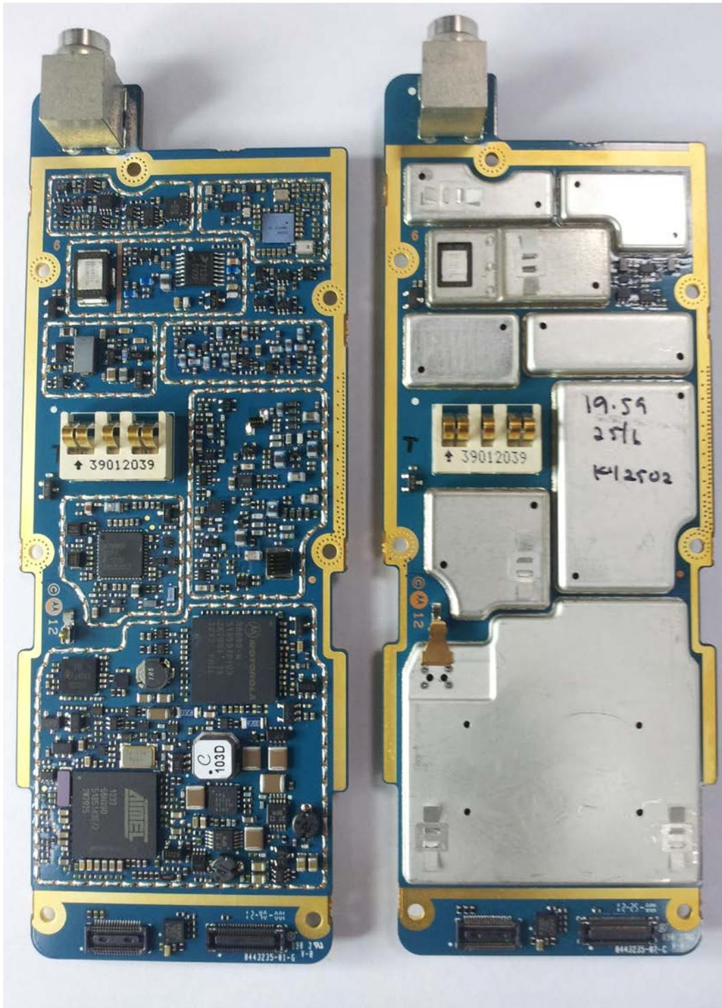
RF board without & with Shields (Bottom)
