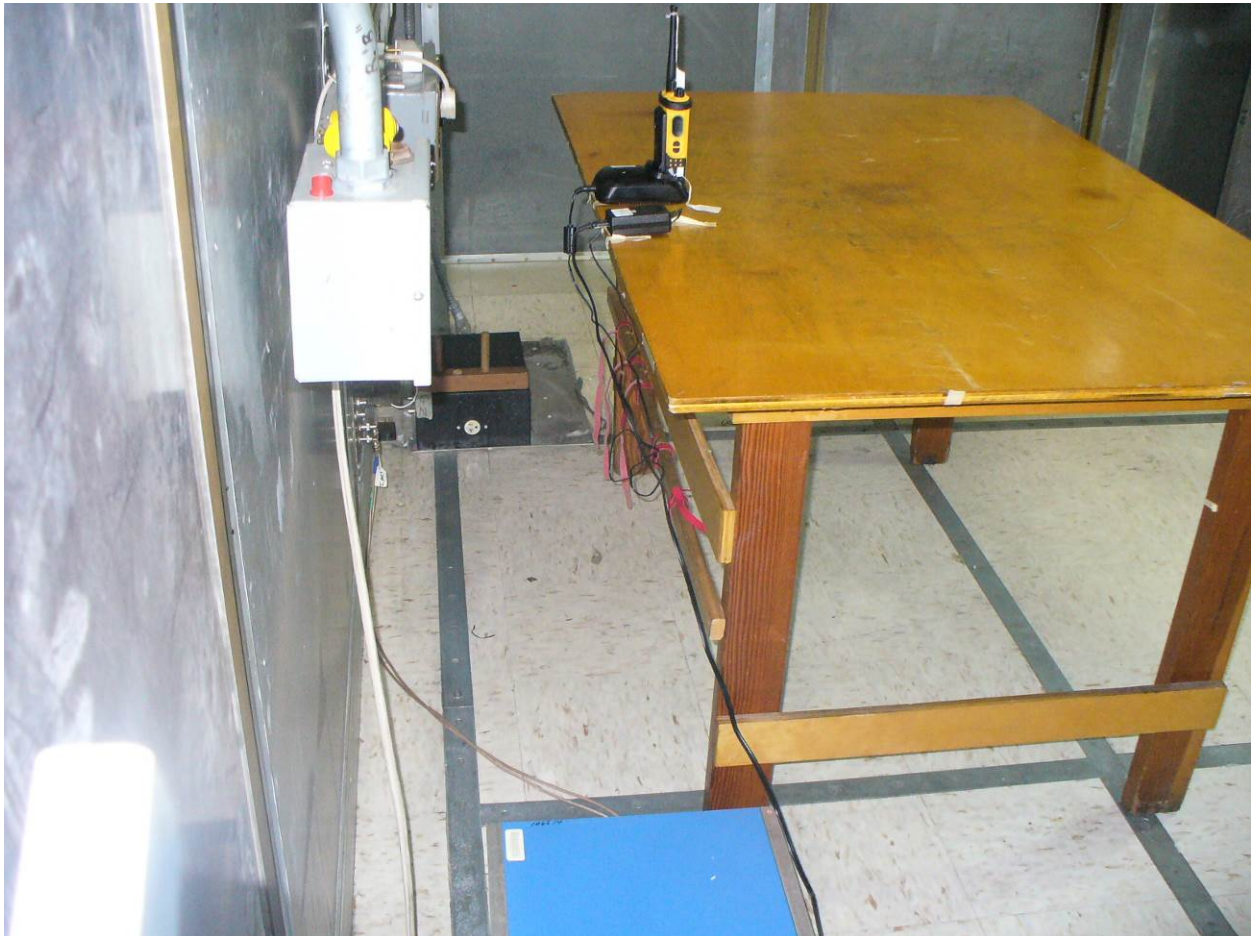
Figure 9: Power Line Conducted Emissions – Side View
