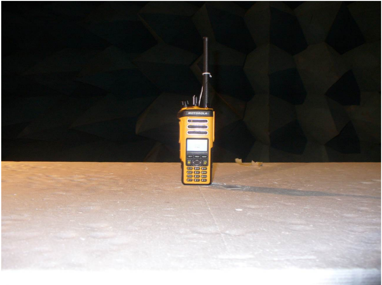
Figure 1: Radiated Emissions – Front View – EUT Standing
