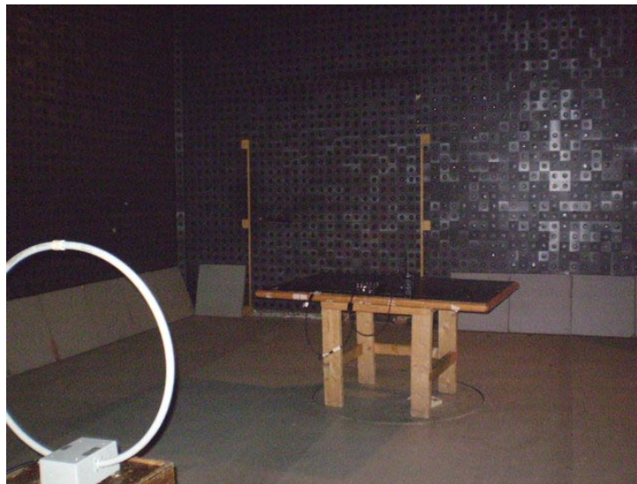
Photograph 7.1.1 Setup for spurious emission field strength measurements in 9 kHz to 30 MHz band
