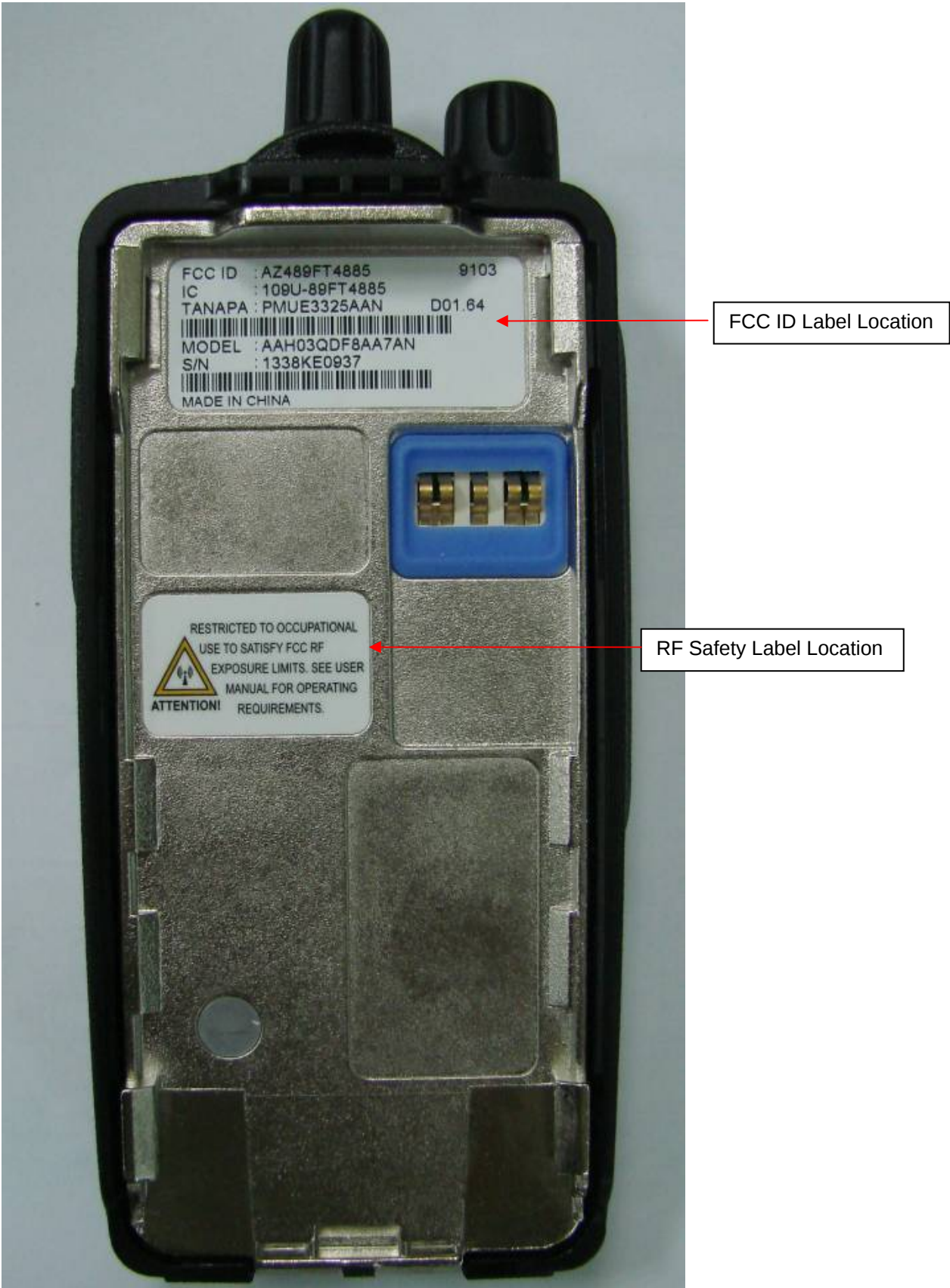
Figure 3-5: Rear view of complete radio showing FCC ID Label & RF Safety Label locations
