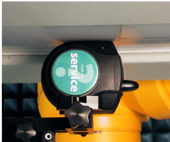
Figure 2: Assessment @ the Body; Right side of DUT against the flat phantom
