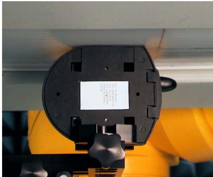
Figure 3: Assessment @ the Body; Left side of DUT against the flat phantom
