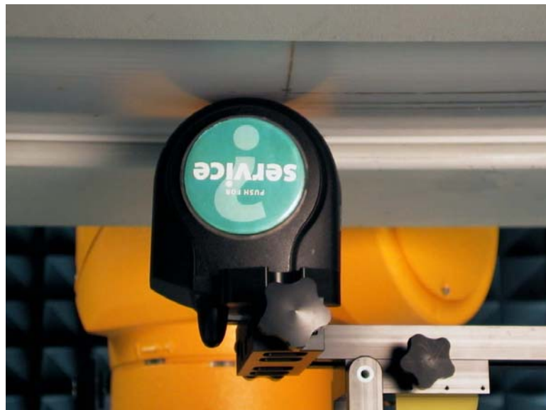
Figure 4: Assessment @ the Body; Bottom side of DUT against the flat phantom
