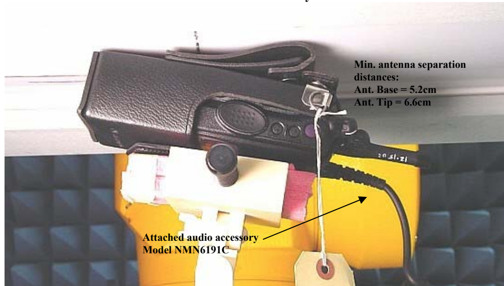
Figure 5. Assessment @ the body. DUT with carry case accessory model NTN8382B against the phantom With attached audio accessory model NMN6191C
