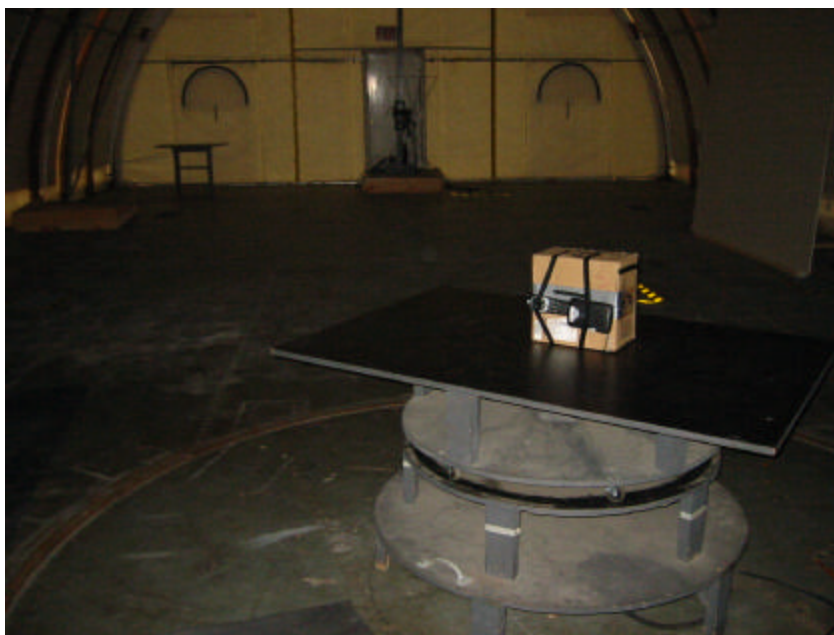
Transmitter Spurious Test Setup, Front View
