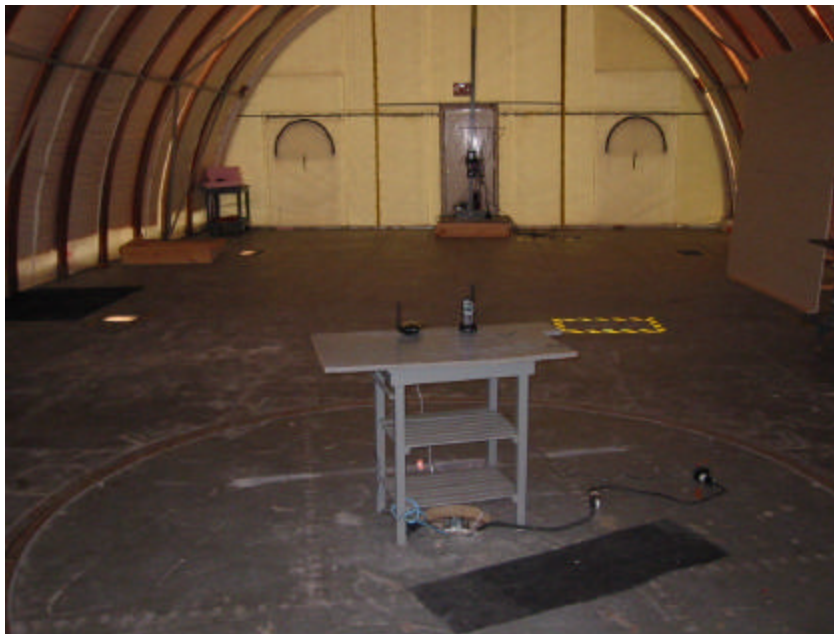
Unintentional Radiator Spurious Test Setup, Front View
