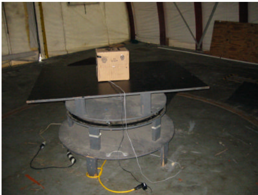
Transmitter Spurious Test Setup, Back View
