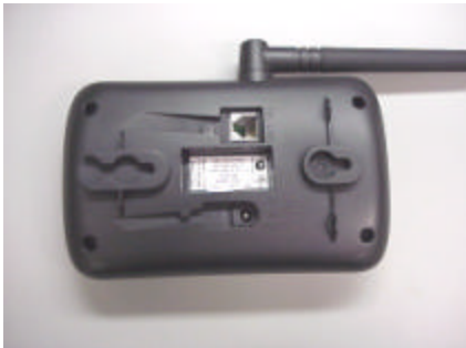
Rear view of Base.
