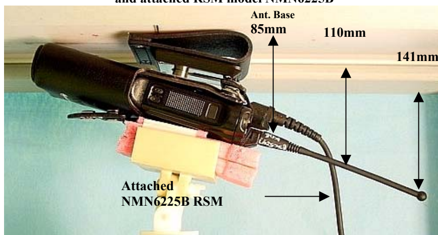
Figure 4. Assessment @ the Abdomen; DUT w/ carry case accessory model NTN5644ASP01/ belt loop model 4205633T01 & NTN5574ASP02 NYPD-T strap, and attached RSM model NMN6225B
