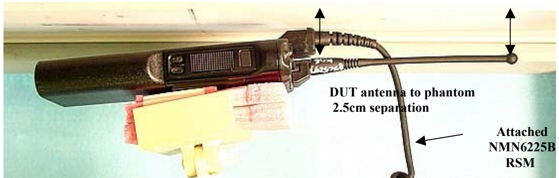
Figure 5: Assessment @ the Abdomen; DUT back towards the phantom and antenna separated 2.5cm, w/ attached RSM model NMN6225B
