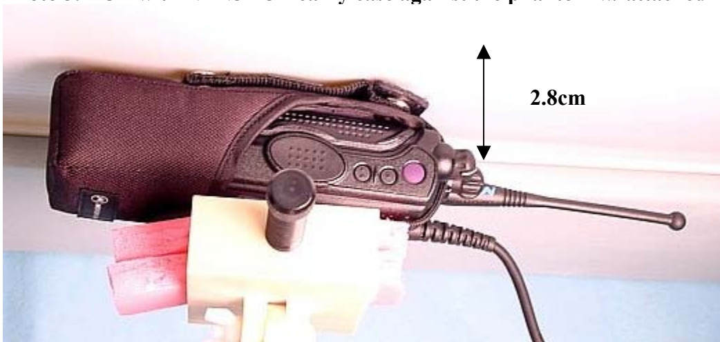
Photo 3. DUT with NTN8725A carry case against the phantom w/ attached RSM
