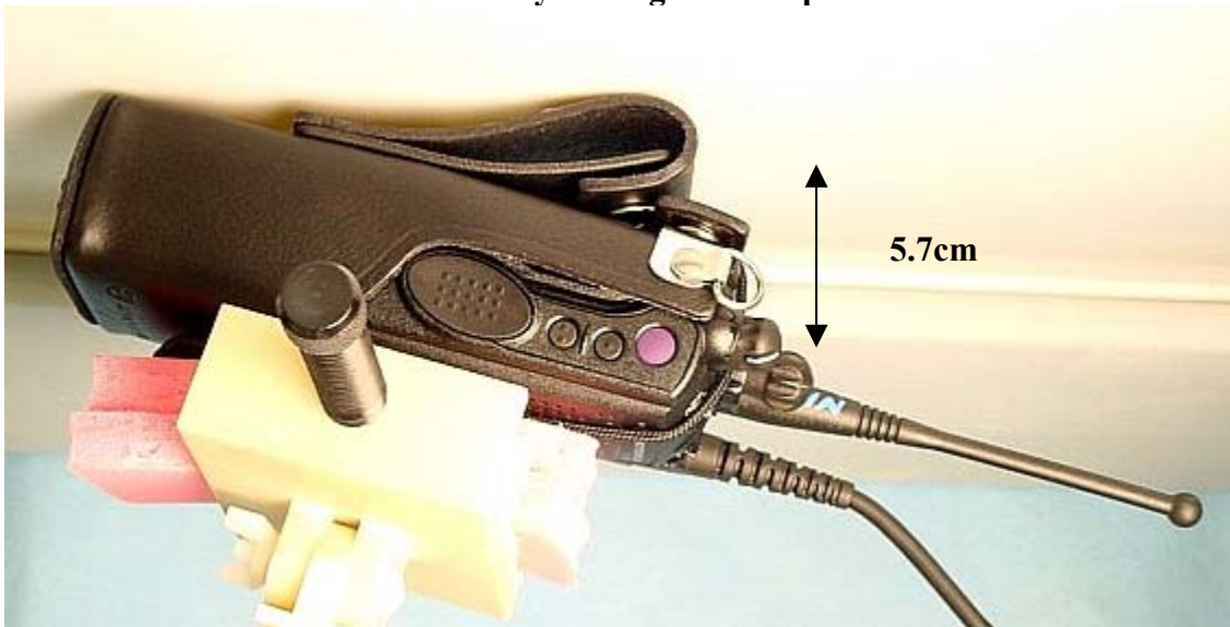
Photo 2. DUT with NTN8387A carry case against the phantom w/ attached RSM
