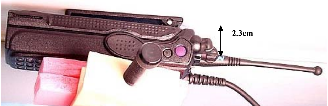
Photo 7. DUT with NTN8460A carry case against the phantom w/ attached RSM
