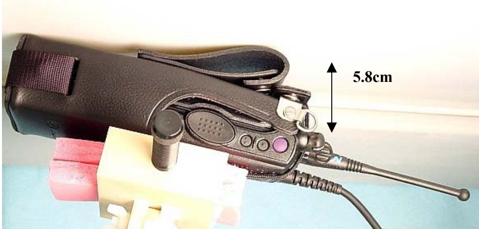
Photo 5. DUT with NTN9184A carry case against the phantom w/ attached RSM
