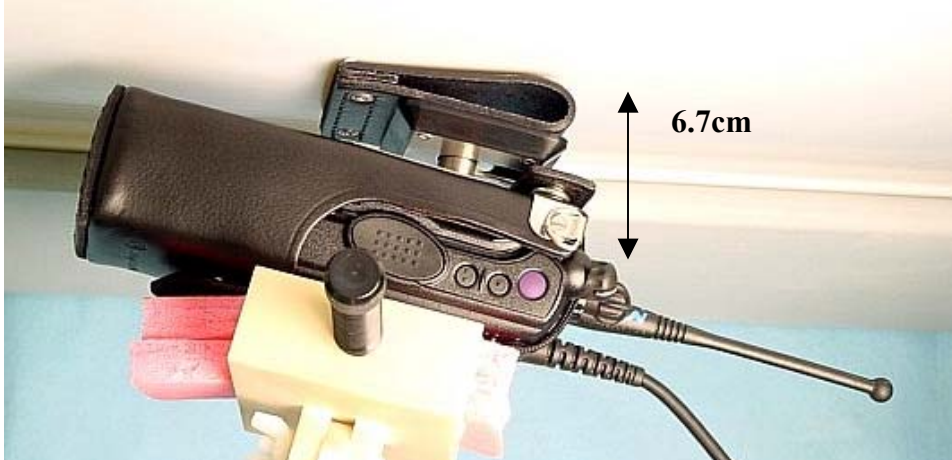
Photo 1. DUT with NTN8380B carry case against the phantom w/ attached RSM
