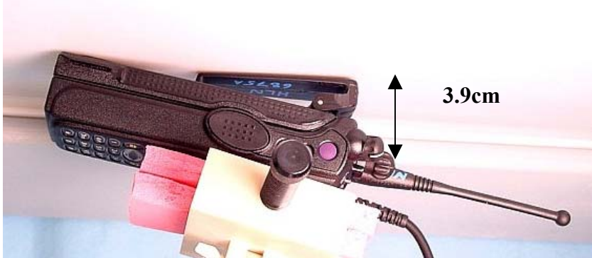
Photo 1. DUT with HLN6875A belt clip against the phantom w/ attached RSM
