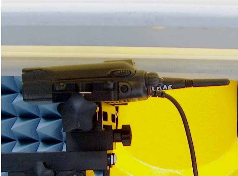
Figure 3: Body Assessment DUT back housing w/ antenna separated 2.5cm from the phantom Worst case audio acc. Model HMN9052E attached
