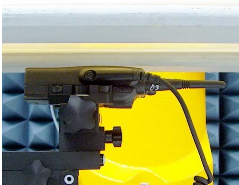
Figure 4: Body Assessment DUT w/ front housing separated 2.5cm from the phantom Worst case audio acc. Model HMN9052E attached
