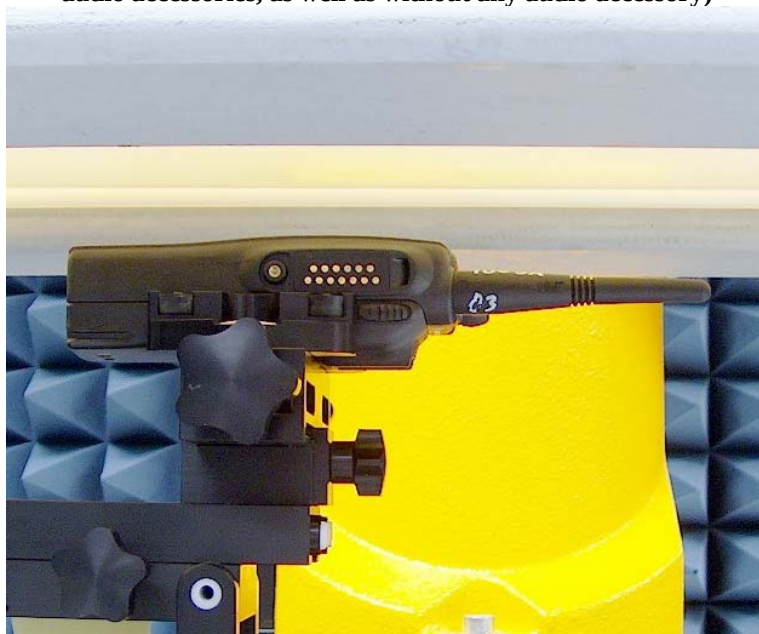
Figure 2: Highest S.A.R. Test Position (face); Antenna PMAE4003A DUT front side separated 2.5cm from the phantom (same position used for other offered antenna, all other applicable audio accessories, as well as without any audio accessory)
