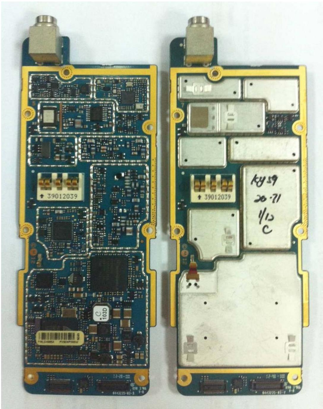
RF board without & with Shields (Bottom)
