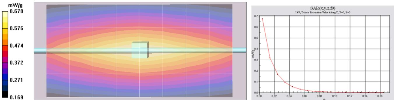
**DIPOLE SAR TARGET - HEAD**
