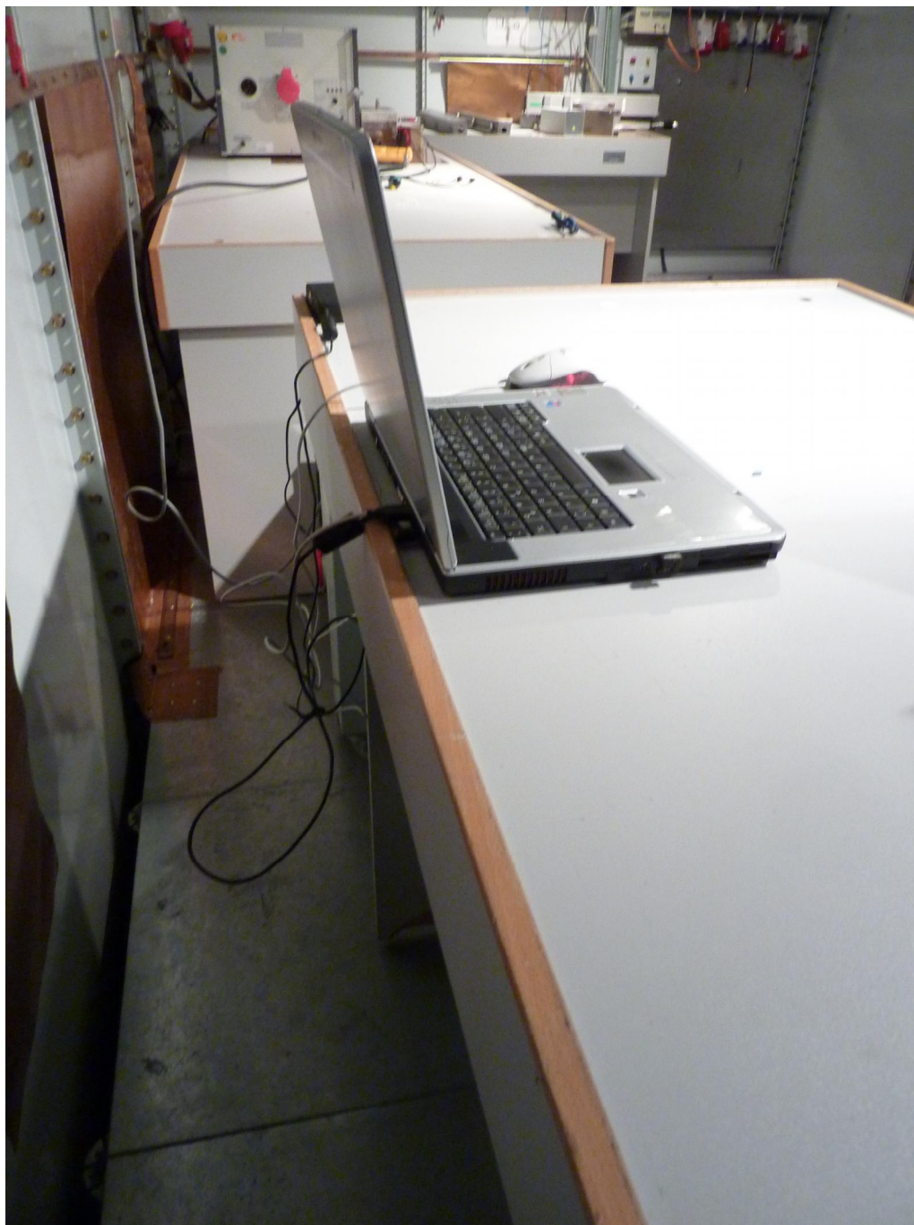
121150_17: Test set-up: Conducted emissions on power supply lines
