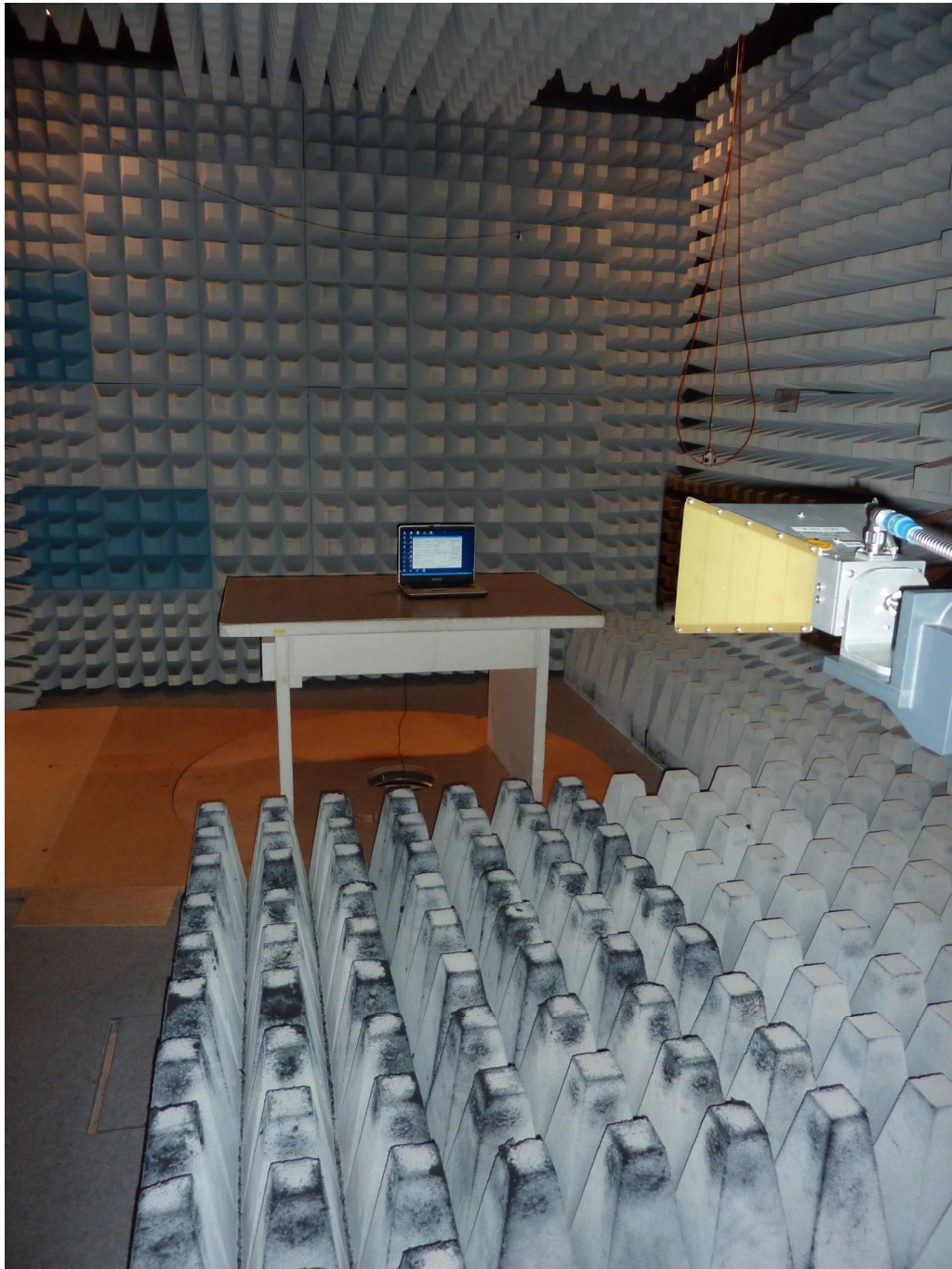
121150_3: Test set-up: fully anechoic chamber (Preliminary & Final measurement 1 GHz – 12 GHz)
