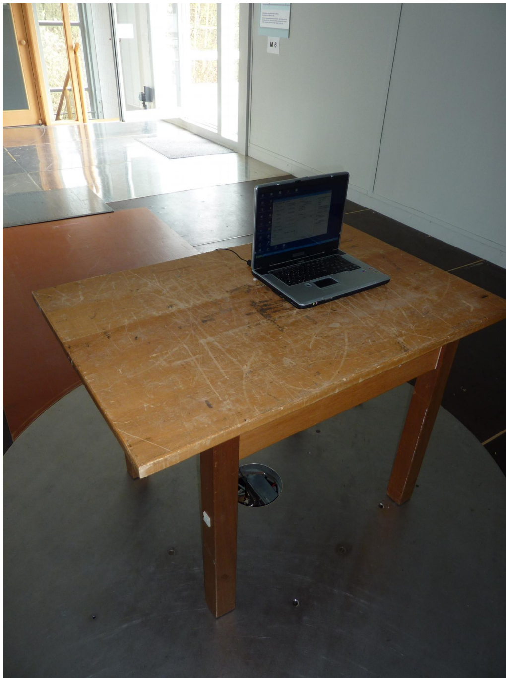
121150_16: Test set-up: open area test site (Final measurement 30 MHz – 1 GHz)
