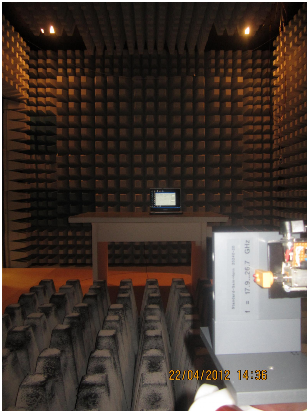
121150_22: Test set-up: fully anechoic chamber (Preliminary & Final measurement 18 GHz – 22 GHz)
