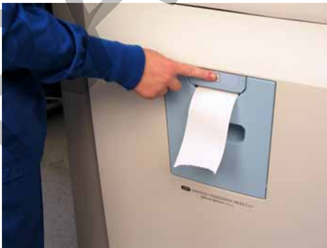
Figure 32. Press the Paper Advance Button.
