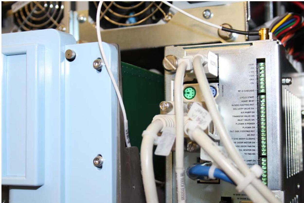
Picture showing RFID Antenna inside the EUT (RFID module inside the Controller box)
