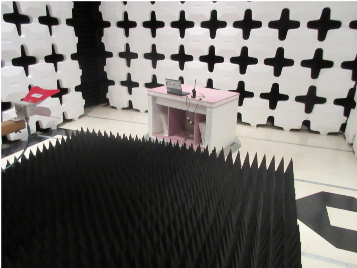
AC Powerline Conducted Final Setup
