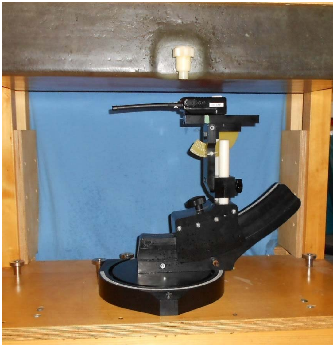
Face-held SAR Configuration Test Setup
