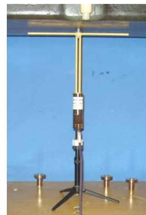
SPEAG 450 MHz Validation Dipole Setup
