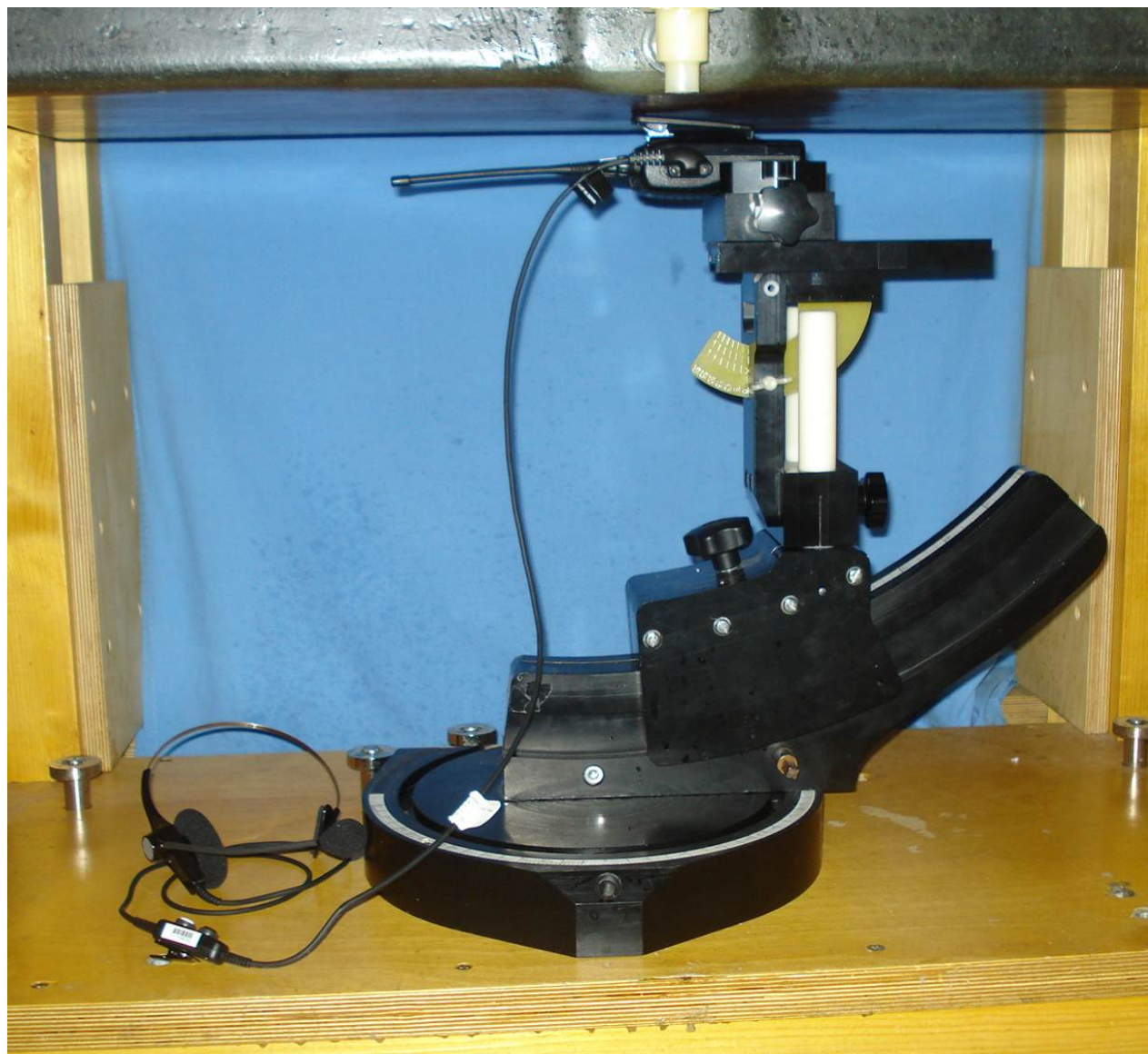
Body-worn SAR Configuration Test Setup
