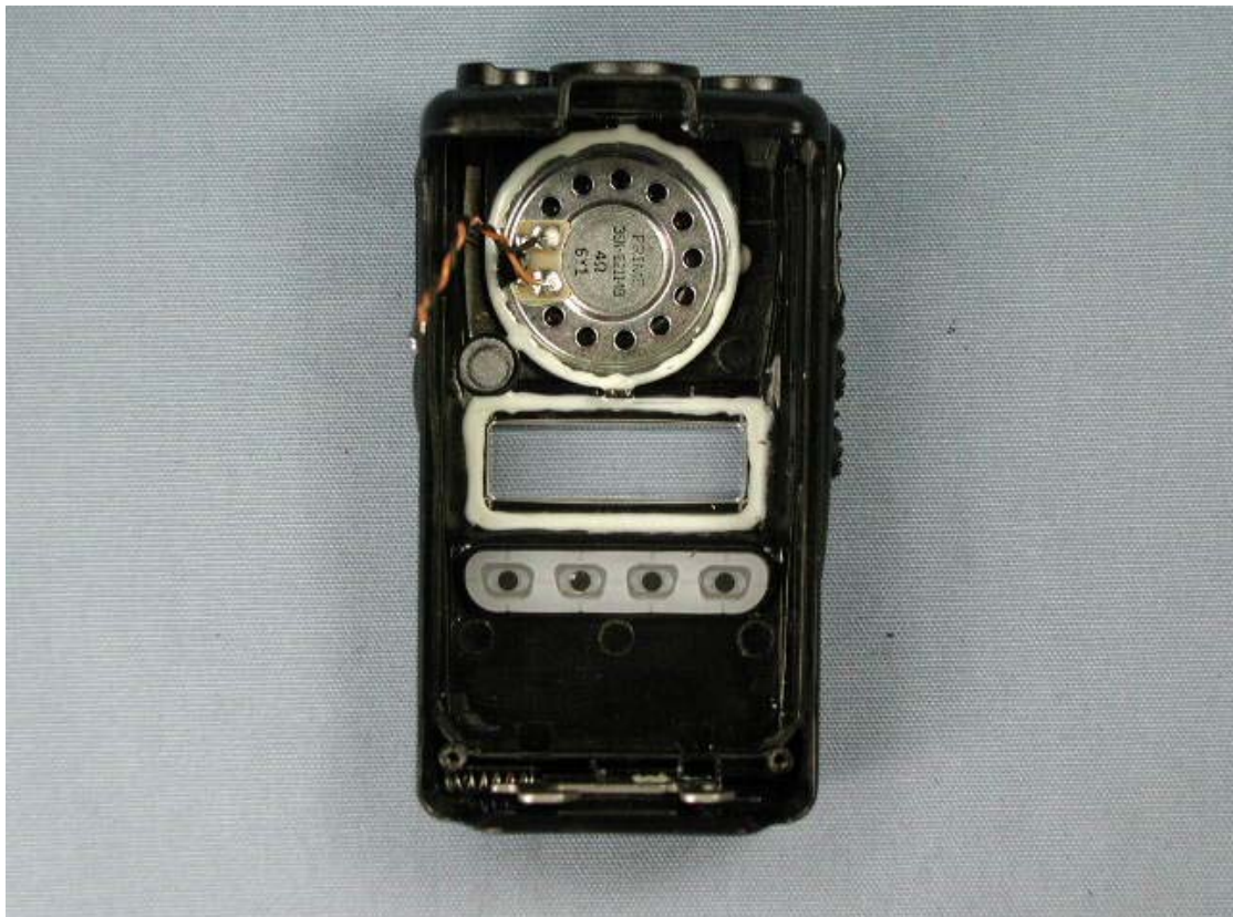
Inside of front panel (for VX-354)
