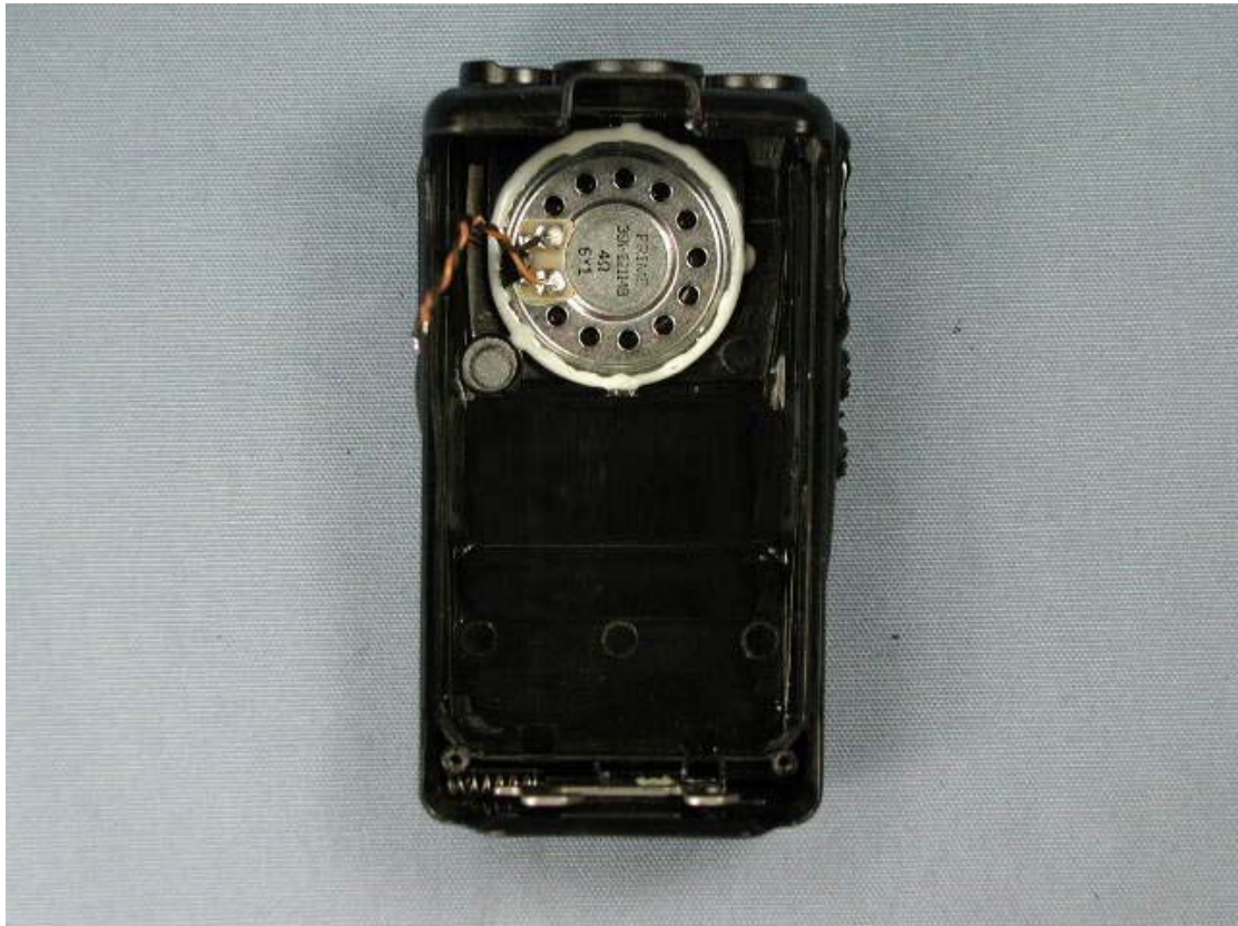
Inside of front panel (for VX-351)
