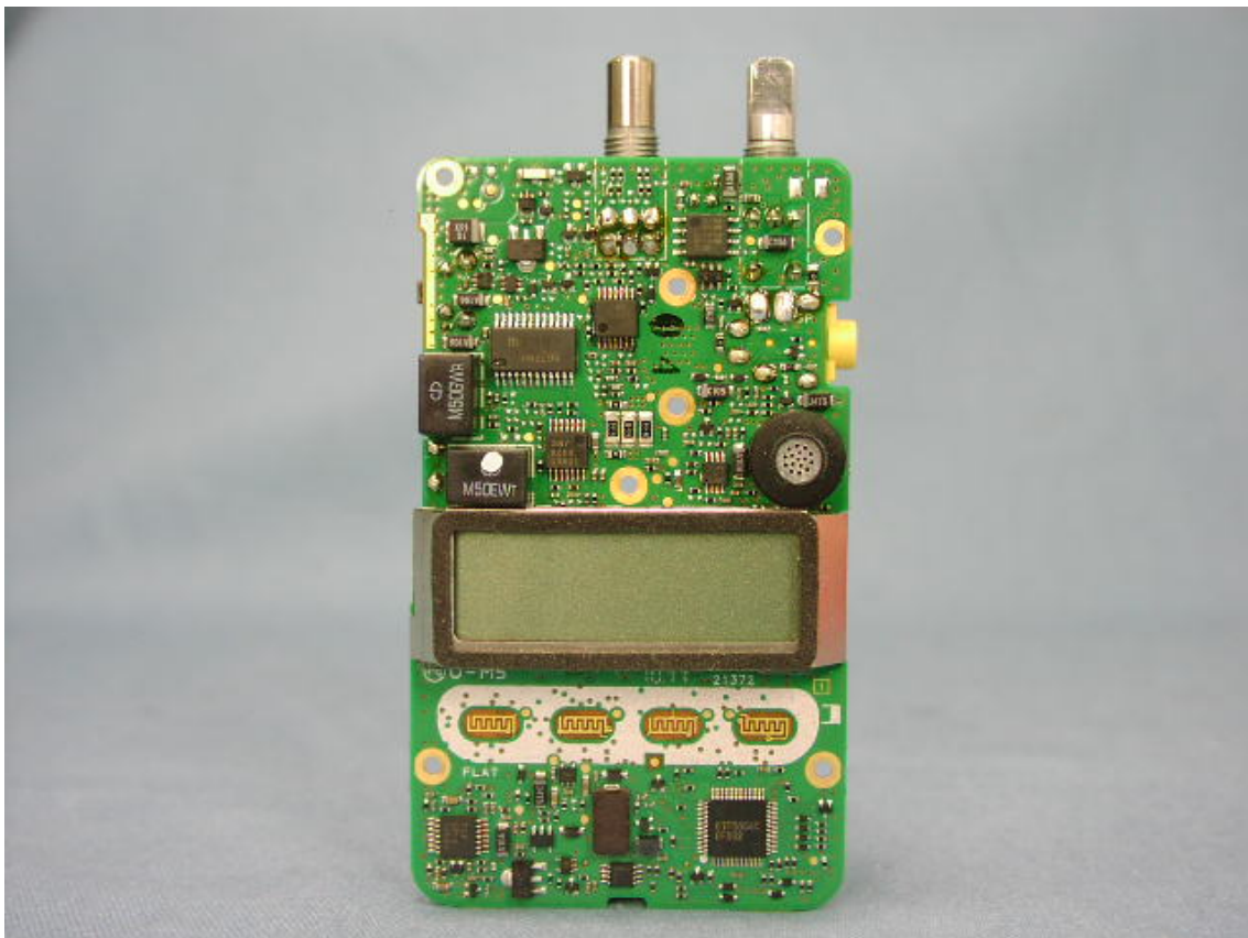
Side-A of MAIN-5-UNIT with LCD
