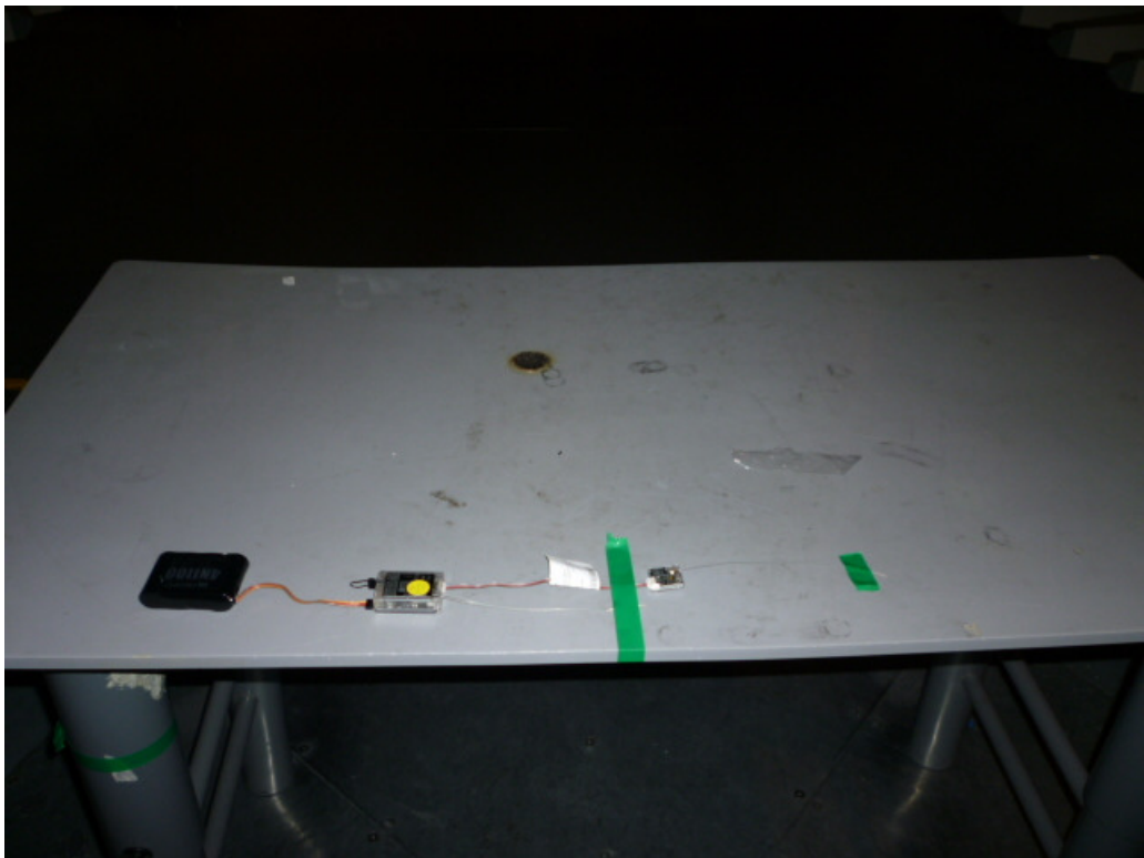
Set-up for Radiated Emission (Transceiver)
