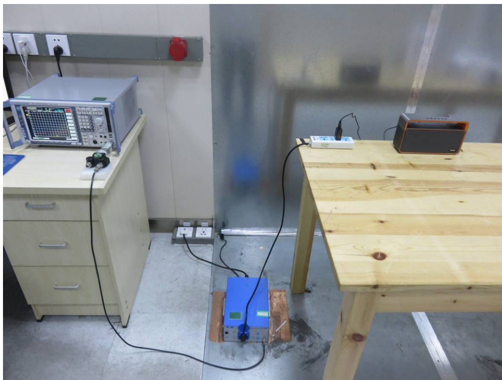
FCC RADIATED EMISSION TEST SETUP
