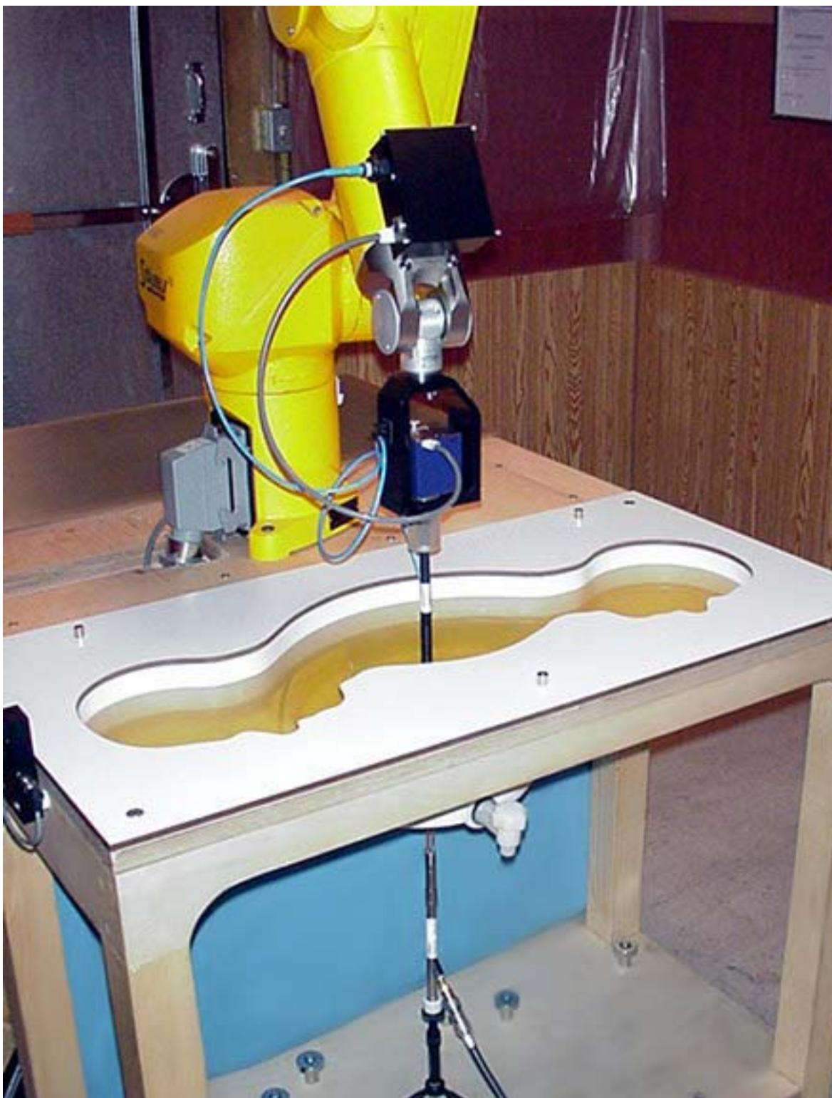
**6. 835 MHz Validation Dipole Setup**
