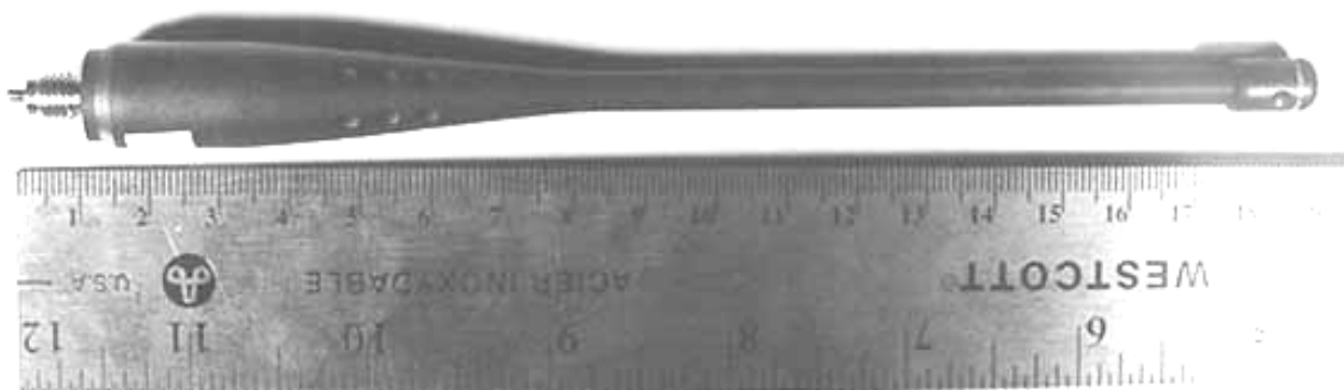
1/2-Wave Antenna (P/N: KRE 1011 506/1)
