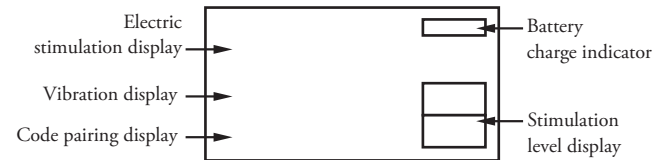
figure 7 – LCD Display Window on Remote Transmitter
