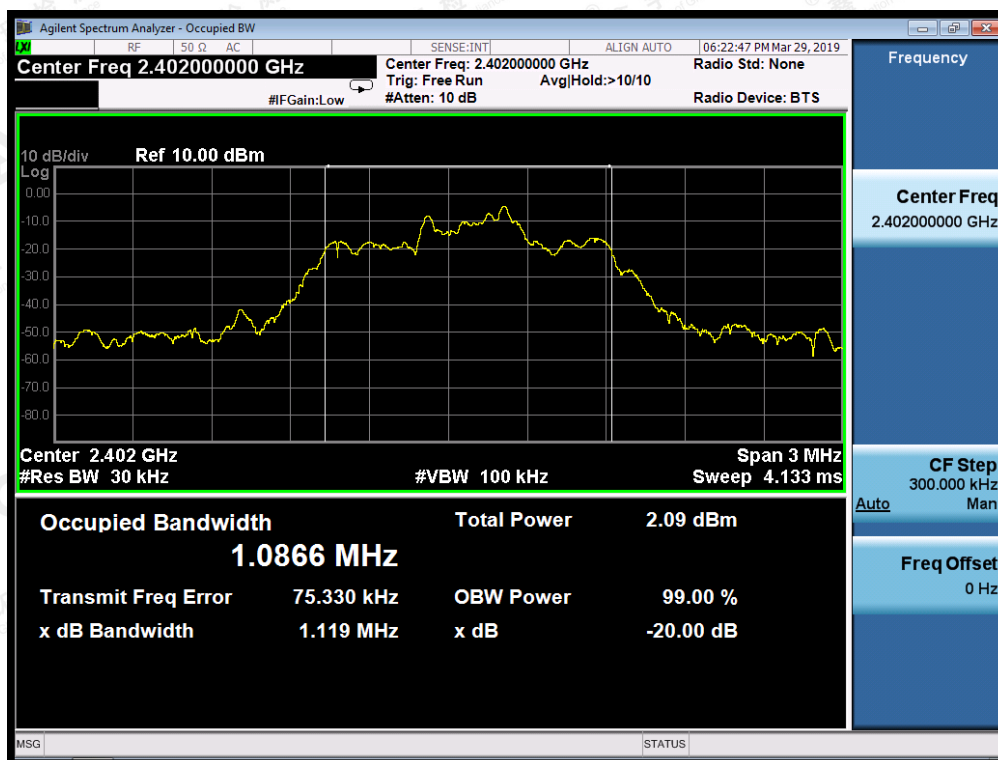
TEST PLOT OF BANDWIDTH FOR LOW CHANNEL
