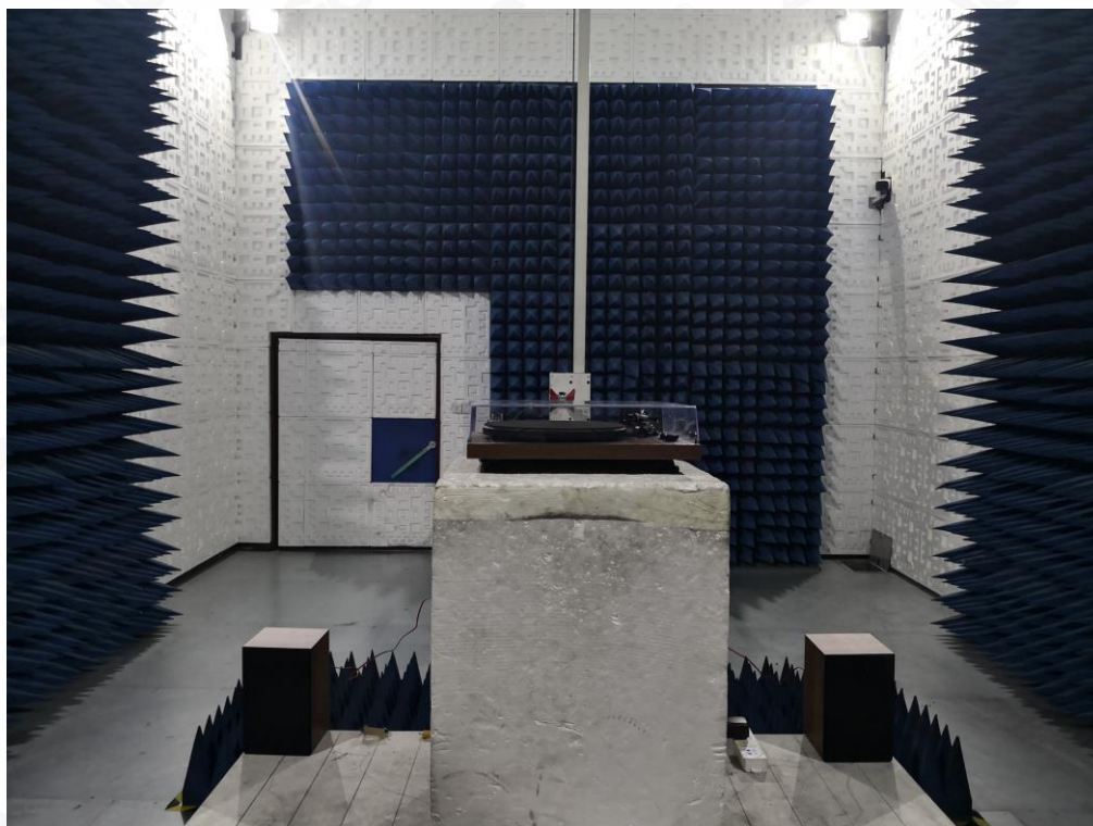
RADIATED EMISSION TEST SETUP ABOVE 1GHZ
