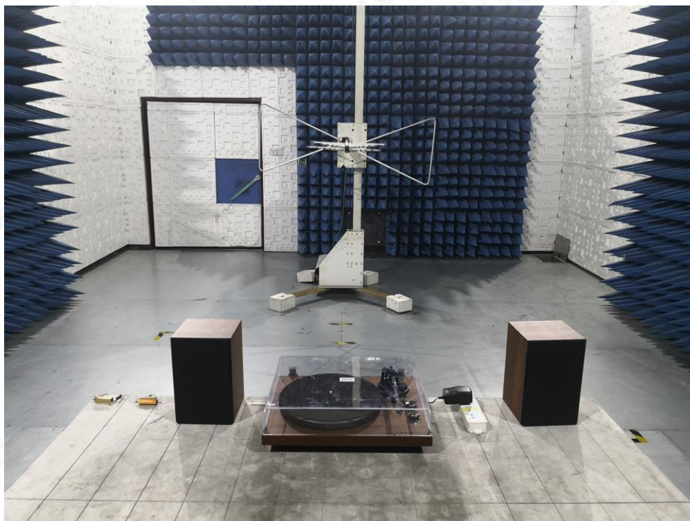
RADIATED EMISSION TEST SETUP ABOVE 1GHZ
