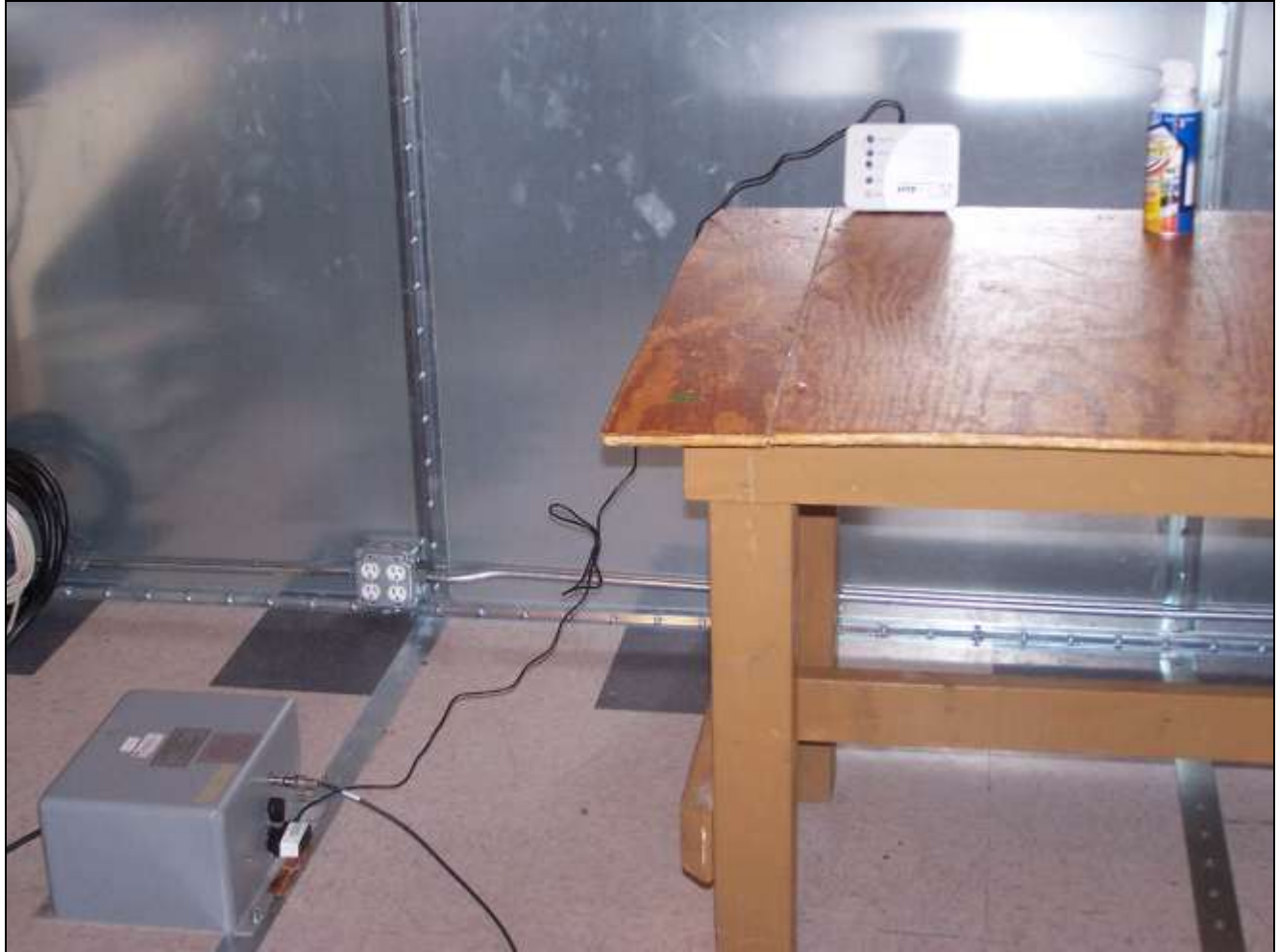
Photograph 1. Conducted Emissions, Test Setup
