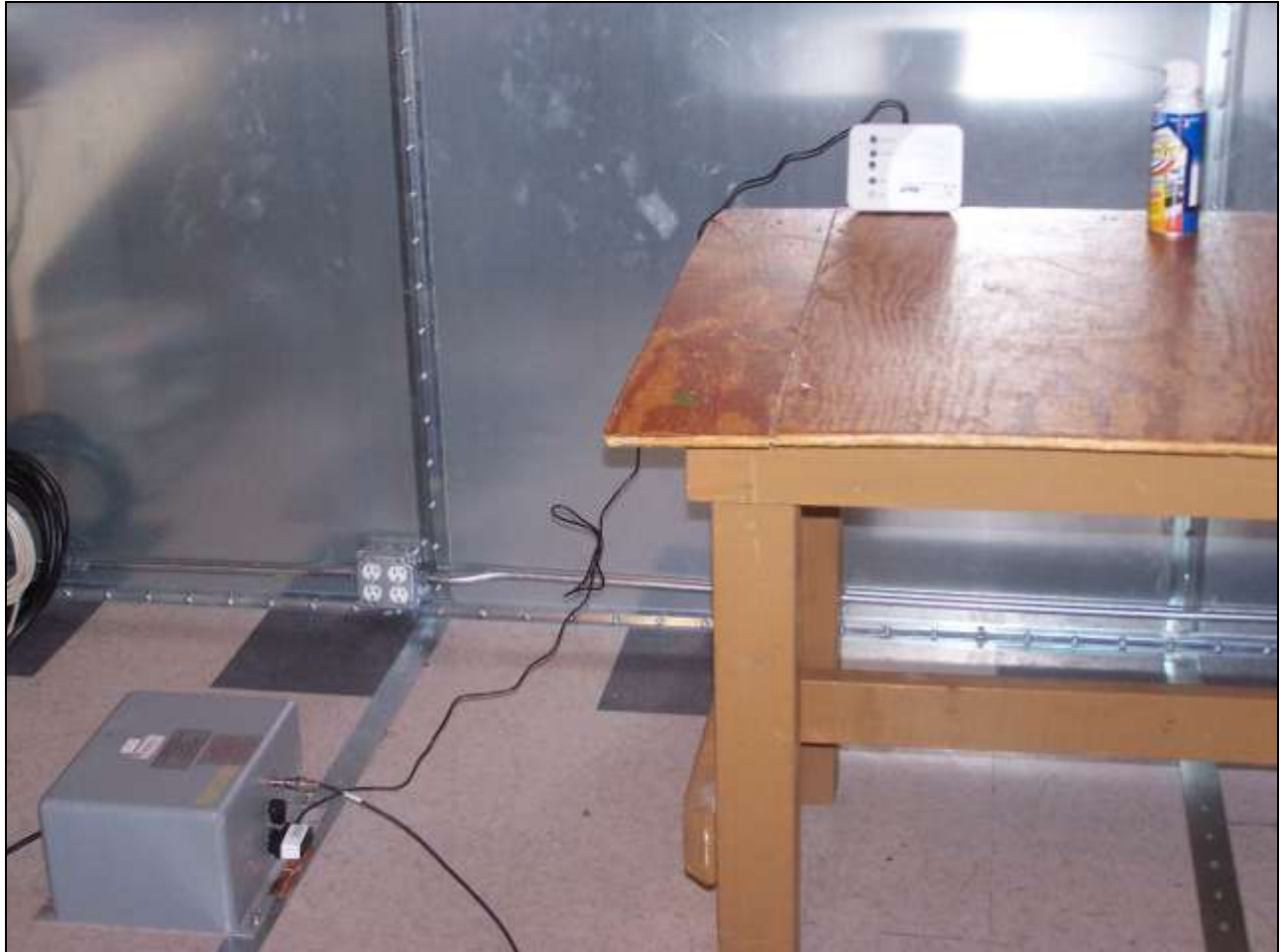
Photograph 4. Conducted Emissions, 15.207(a), Test Setup
