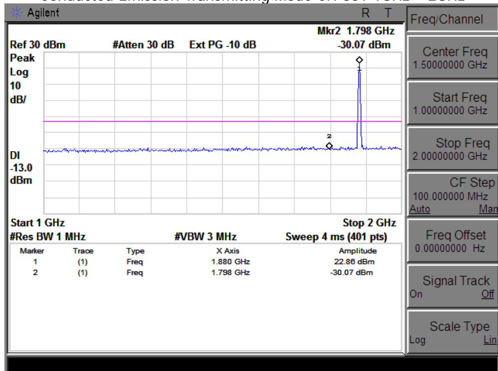
Conducted Emission Transmitting Mode CH 661 2GHz – 20GHz
