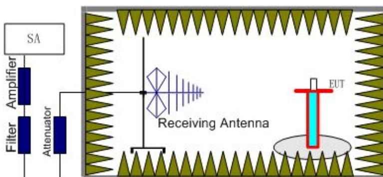
Radiated emissions measurements were made only at the upper, middle, and lower carrier frequencies of the PCS1900 band (1850.2 MHz, 1880 MHz and 1909.8 MHz), GSM850 band (824.2MHz, 836.6MHz, 848.8MHz). It was decided that measurements at these three carrier frequencies would be sufficient to
