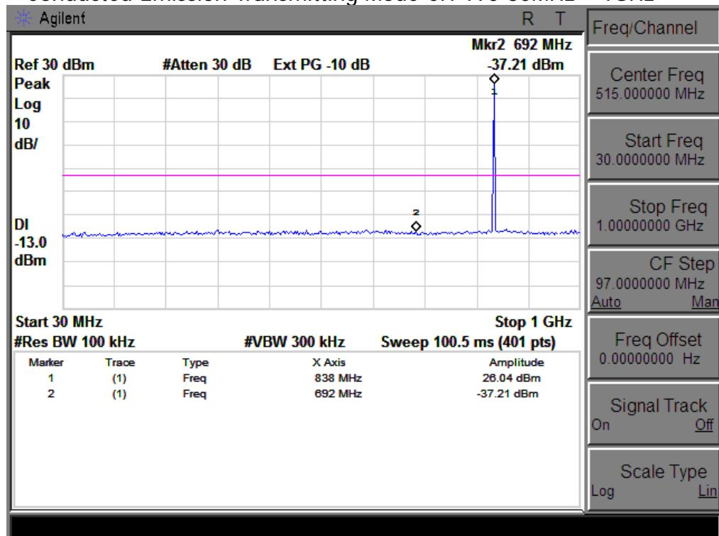
Conducted Emission Transmitting Mode CH 190 1GHz – 10GHz
