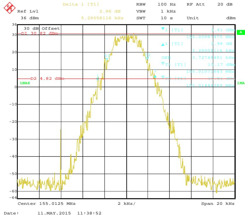
**99% Occupied Bandwidth & 26 dB Emissions Bandwidth 6.25 kHz, 155.0125 MHz (Low Power)**
