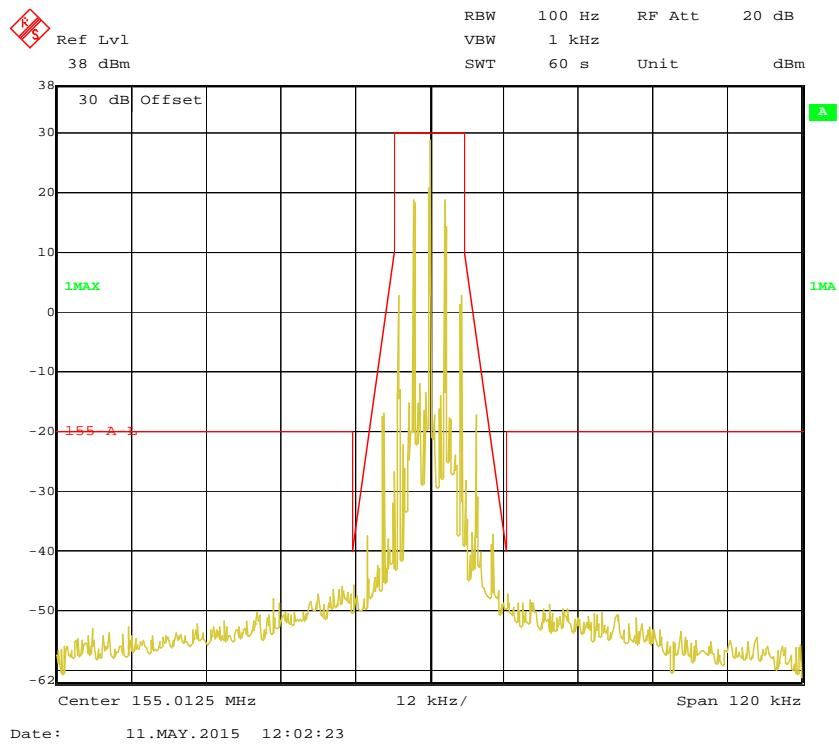
**Digital Modulation:****99% Occupied Bandwidth & 26 dB Emissions Bandwidth 6.25 kHz, 155.0125 MHz (High Power)**
