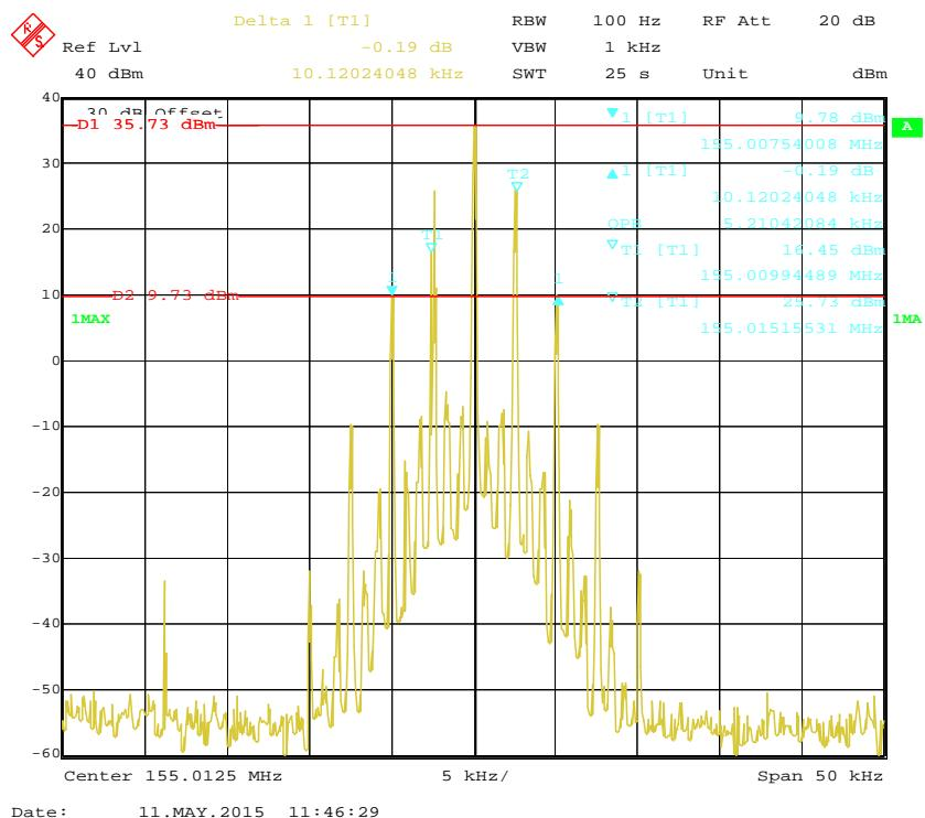
**99% Occupied Bandwidth & 26 dB Emissions Bandwidth 12.5 kHz, 155.0125 MHz (Low Power)**
